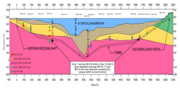
Figure 4: Hydraulic Conductivity along proposed alignment
