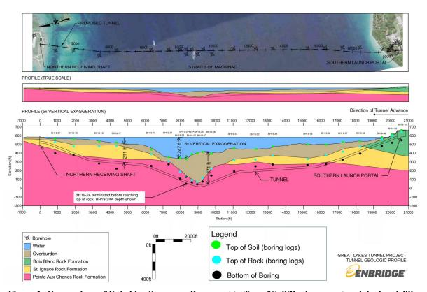
Figure 1: Comparison of Enbridge Summary Document to Top of Soil/Rock encountered during drilling
