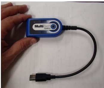
COTS mobile broadband modem with USB connectivity. Available for both CDMA and GSM carriers.
