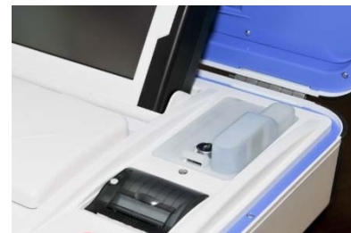
Verity Scan's vDrive/USB/Modem compartment, closed and locked.
