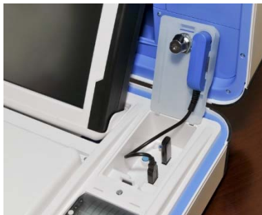
Verity Scan's vDrive/USB/Modem compartment, open, showing modem with USB connection and vDrive.
