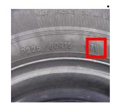
Be certain the tire speed ratings meets or exceeds the speed capability of the vehicle on which the tire is being used. Note: A spinning tire can attain a speed twice the speedometer reading.
