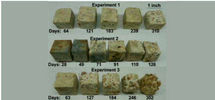
Photo of concrete cubes placed in sewage pipes via Mark Hernandez
