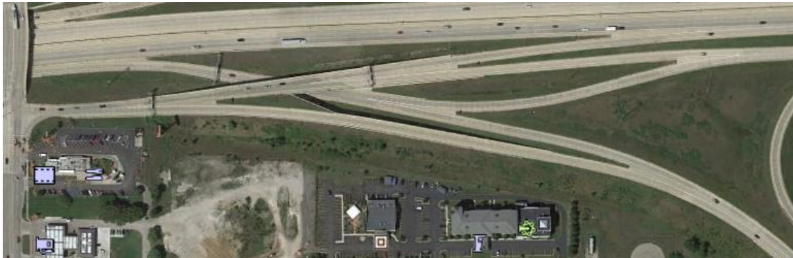
Figure 4.10.1 – Example of Ramp “Braiding”
