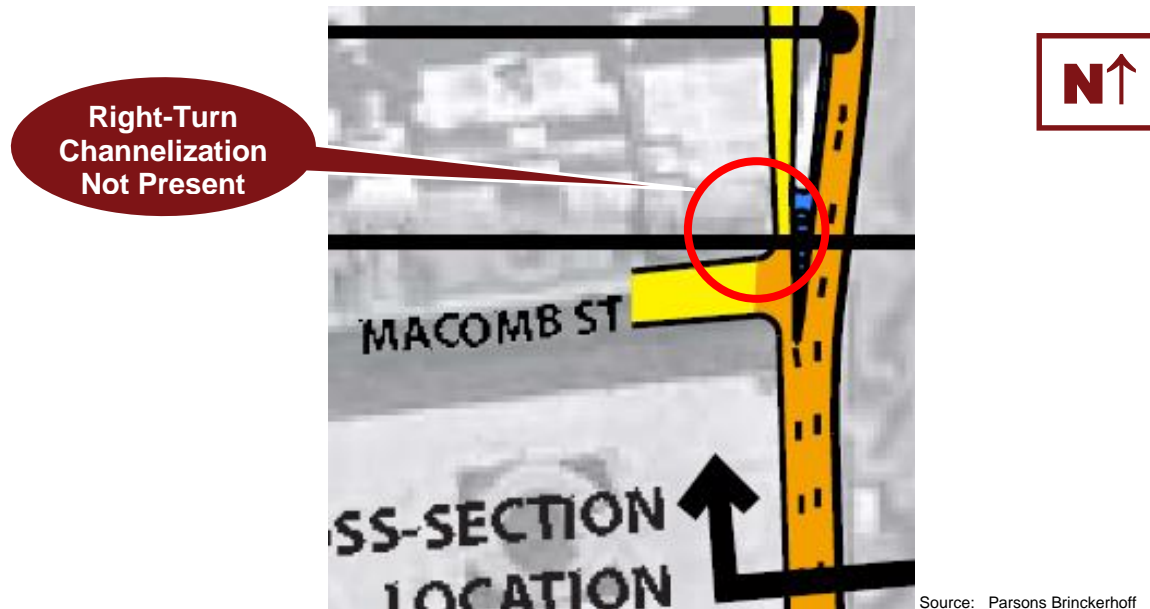
Figure 5.2.3.1 – Right-Turn Channelization Not Present
