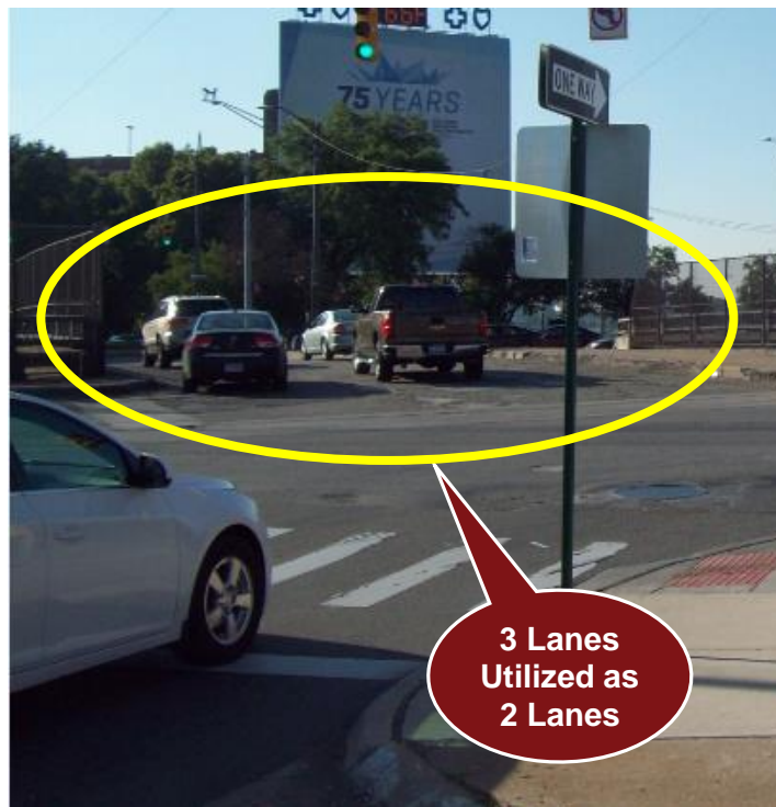
Figure 4.13.1 – SB Chrysler Drive to EB Jefferson Ave Lane Usage
