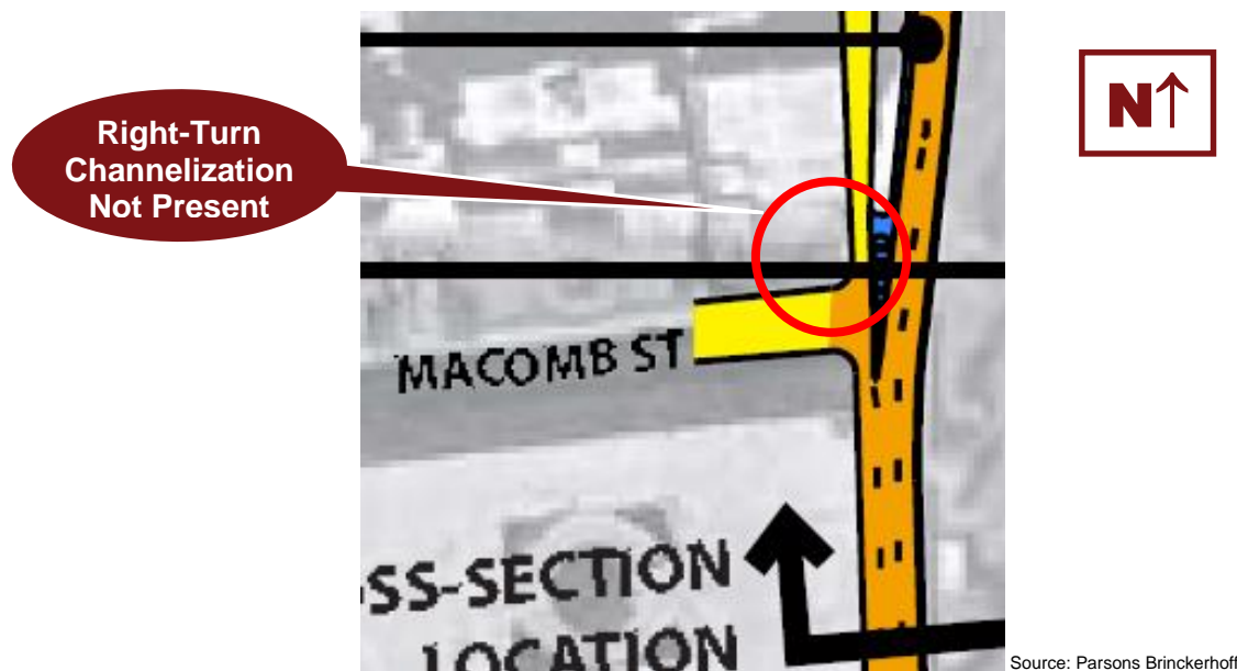
Figure 5.1.3.1 – Right-Turn Channelization Not Present
