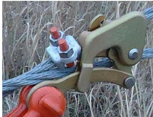
Safety latches on cable grips help keep the cable grip from slipping off the cable. As an additional precaution, securing a c-clamp to the safety latch will help keep the safety latch in place and reduce the chances of the safety latch failing if subjected to a large lateral force. Also, attaching a u-bolt cable clamp to the cable, directly behind the cable grip, will help keep the cable grip from slipping along the cable.
