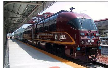
**Diesel Multiple Unit (DMU)**
