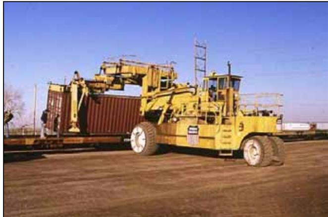
**Intermodal Container Being Loaded to Railcar**
