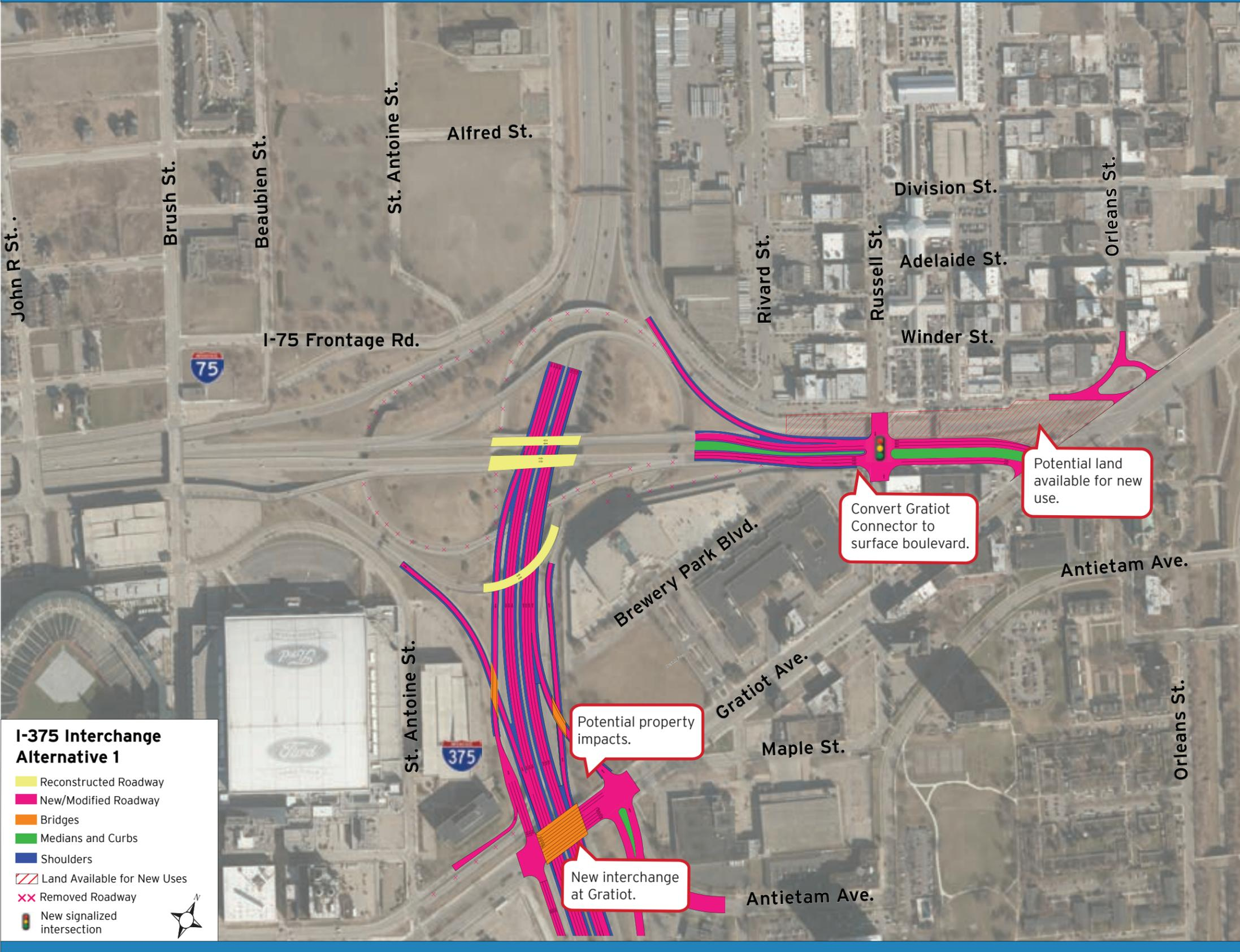
Alternative 1 is intended as a lower-cost upgrade of the interchange area, which would eliminate the current left-hand ramps to Madison Avenue, and create a more traditional interchange at Gratiot Avenue. It would also include conversion of the Gratiot connector to a surface roadway with a signalized intersection at Russell Street. This alternative is compatible with all six of the I-375 alternatives.
