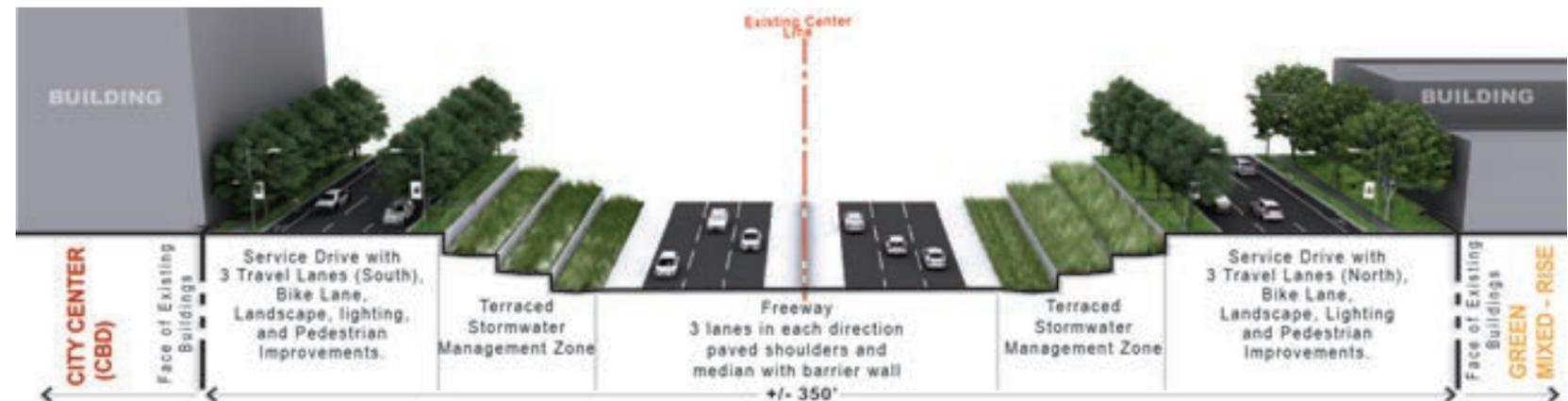
CROSS-SECTION LOOKING NORTH SHOWING PROPOSED CONDITIONS
