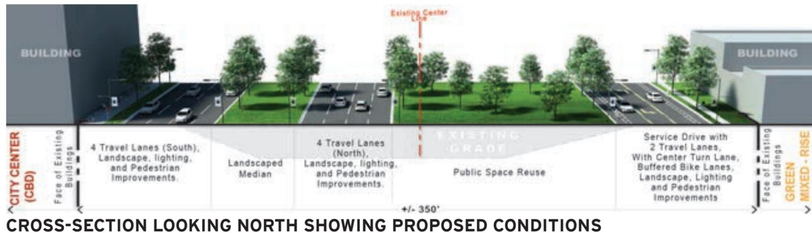
CROSS-SECTION LOOKING NORTH SHOWING PROPOSED CONDITIONS
