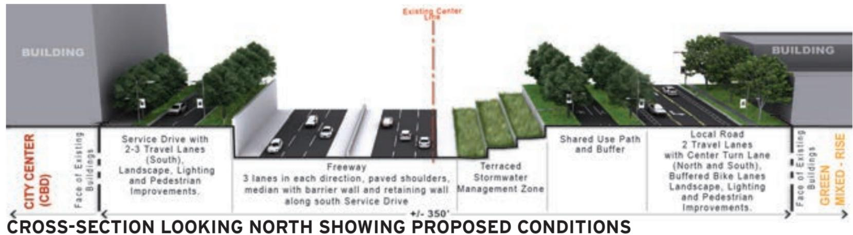
CROSS-SECTION LOOKING NORTH SHOWING PROPOSED CONDITIONS
