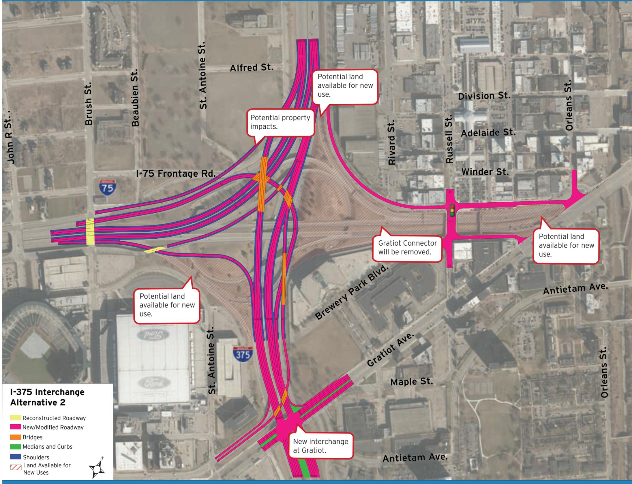
Under Alternative 2, the interchange area would be completely reconstructed, with I-75 reconfigured as the through-traffic movement. A surface street intersection would be created with Gratiot Avenue at I-375, replacing the need for the Gratiot connector and allowing for its elimination. In addition, new access would be created to and from the north on I-75 at Brush Street, and access to Madison Avenue maintained. This alternative is compatible only with I-375 Alternatives 4, 5 and 6.
