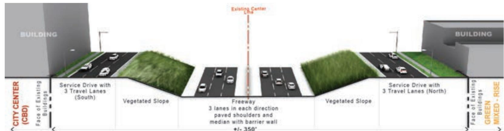
CROSS-SECTION LOOKING NORTH SHOWING PROPOSED CONDITIONS
