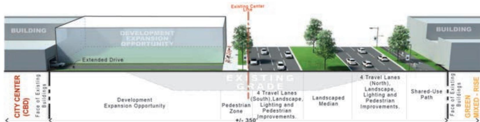
CROSS-SECTION LOOKING NORTH SHOWING PROPOSED CONDITIONS
