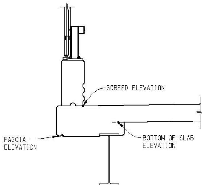
*Figure 1. Screed elevation location at toe of barrier*
