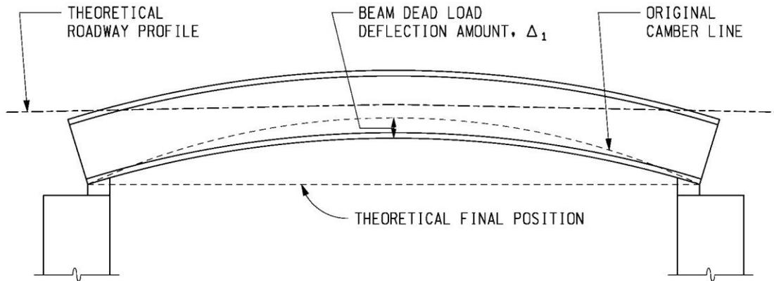
*Figure 4. Deflection of the beam due to self-weight*
