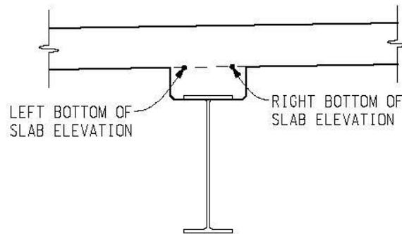
*Figure 2. Bottom of Slab elevation points*
