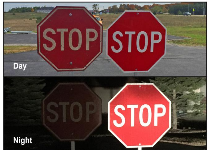
Sign faces on traffic signs are made of reflective sheeting composed of micro-sized prisms
