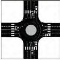
A roundabout is a circular intersection at which all traffic travels counterclockwise, always to the right, around a central island. Vehicles entering from each leg of the intersection must yield to the traffic already in the roundabout, which is coming from the left. Vehicles exit the roundabout by making a right turn onto the desired road.
