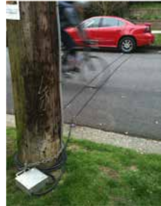
Pneumatic tube counters are inexpensive to set up and maintain, but are not permanently installed.
