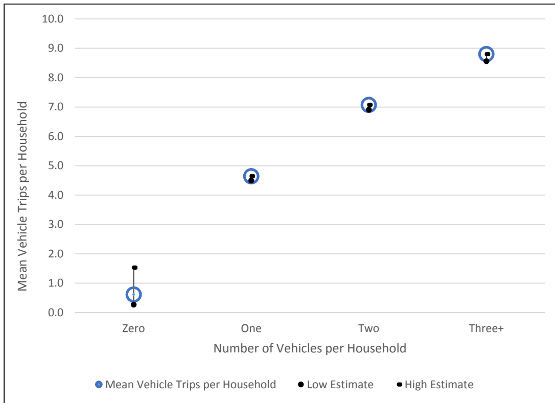
Figure 1-2. Weekday mean vehicle trip rates by number of vehicles in the household, with 95% confidence limits
