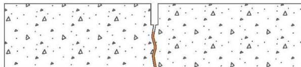
Figure 4. Fine particles infiltrate joint and expansion occurs
