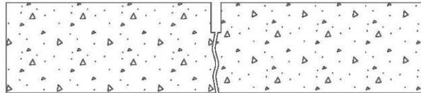
Figure 3. Joint seal lost
