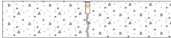
Figure 2. Shrinkage crack forms at contraction joint
