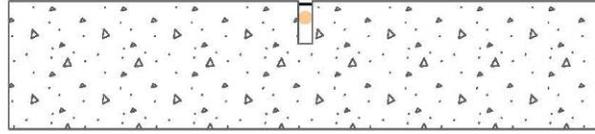
Figure 1. Saw cut and sealed green concrete pavement
