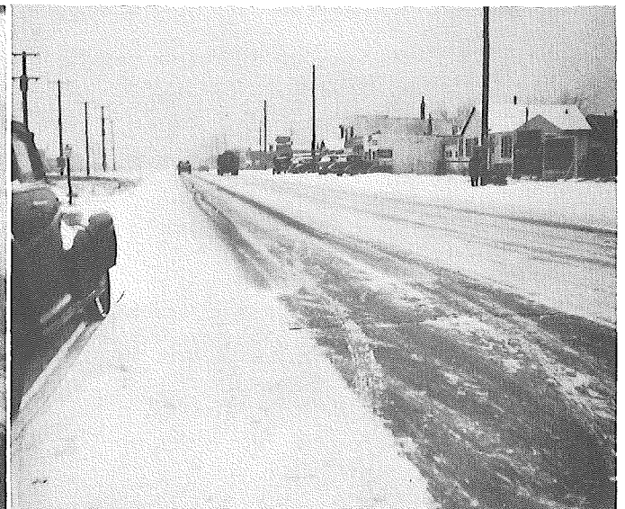
▲ FIGURE 4. CONCRETE SECTION ( 1 - 6 - 50 ) HEATED AREA PARTIALLY CLEARED
