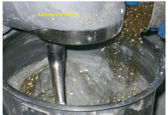
Steel fibers added to the mix help UHPC resist cracking. There is currently only one domestic supplier for steel fibers, but Michigan's manufacturing industry is well-suited to begin offering them if more demand emerges.
