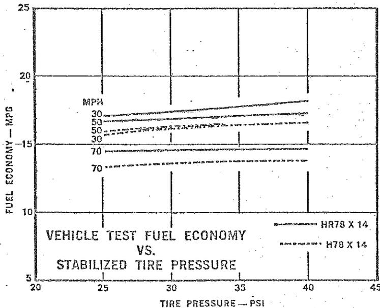
Figure 2 - Vehicle test fuel "economy" versus stabilized tire pressure for radial HR78-14 and bias-belted H78-14 tires.
