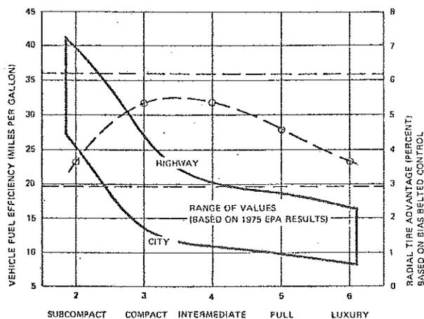
Figure 3. Fuel Efficiency and Radial Tire Advantage by Passenger Car Type.
