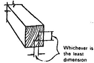
**CHECKS** are measured as an average of the penetration perpendicular to the wide face. Where two or more checks appear on the same face, only the deepest one is measured. Where two checks are directly opposite each other, the sum of their depths is considered.
