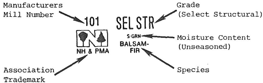
This provides assurance that the material is of a certain quality and that the design stresses can be used with confidence. The use of grade stamped material should correct existing problems in guardrail post procurement. The stamp will also assure that the species is from among the approved list. The use of grade stamps from an approved agency will put the onus of quality assurance on the supplier, rather than on the treating plant or MDOT personnel.
