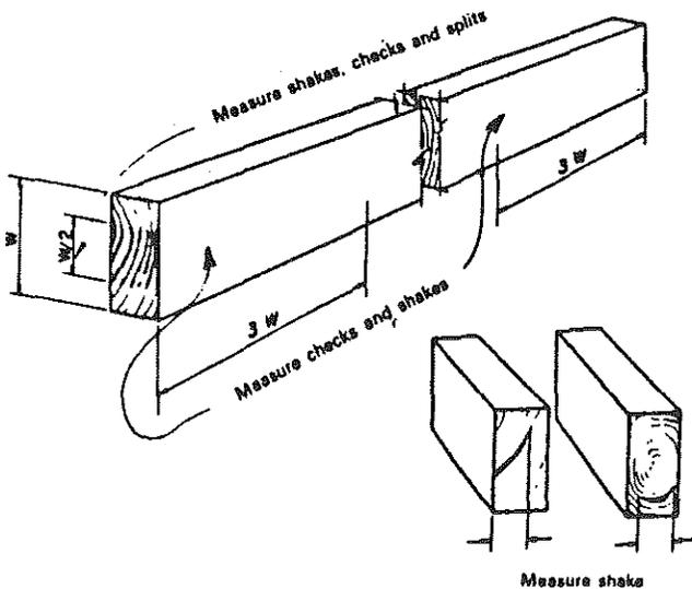
**SHAKES** in Posts and Timbers are measured at the ends of pieces between lines parallel with the two faces that give the least dimension.
