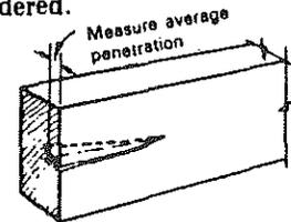
**SPLITS** are measured as the penetration of a split from the end of the piece and parallel to the edges of the piece.
