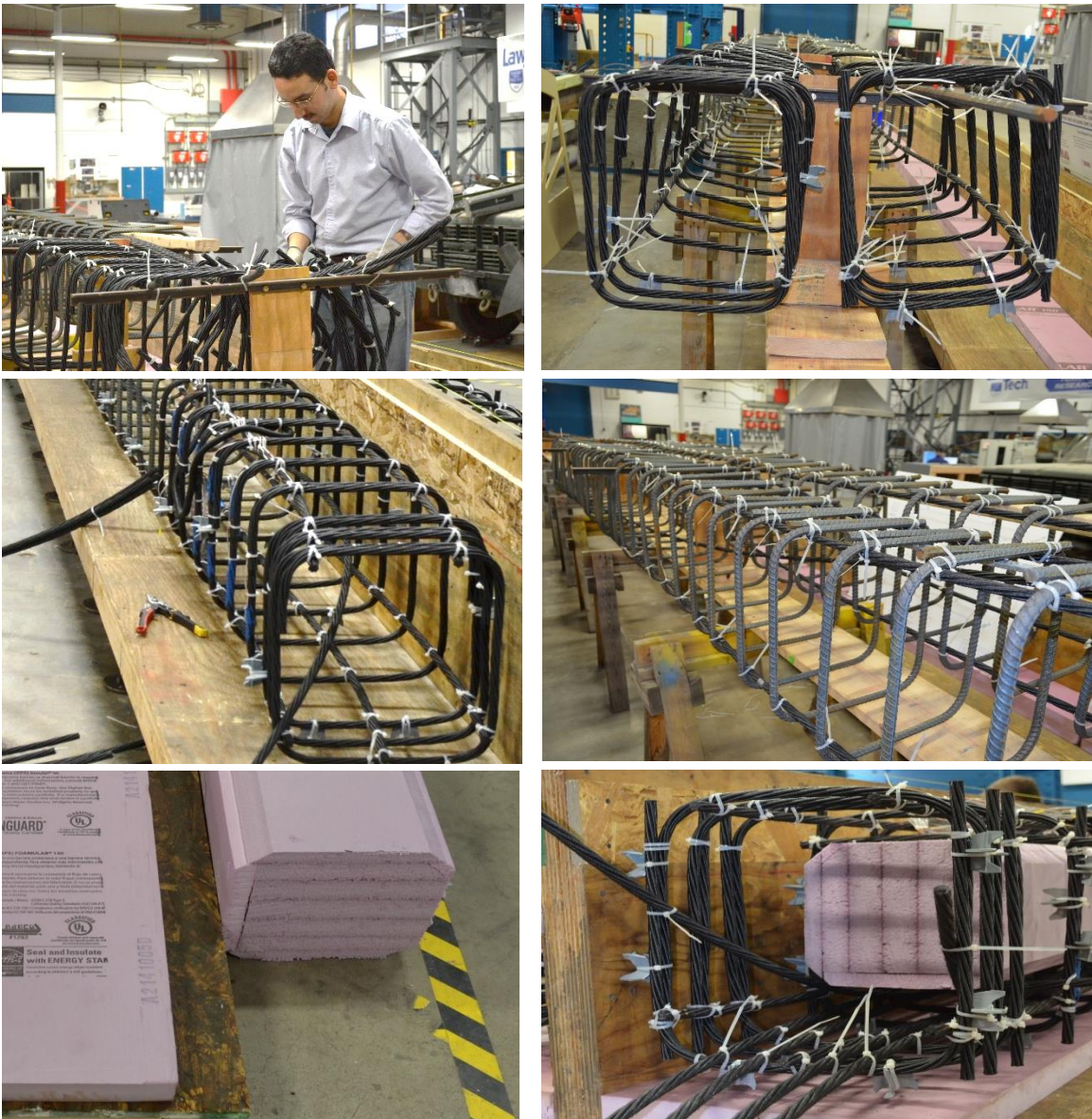
Figure 7.4-7 Preparing and instrumenting the reinforcement cages
