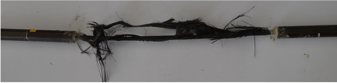
Figure 6.2-7 Failure of CFCC specimen at 482 °F (250 °C)
