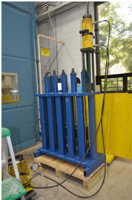
Figure 5.3-2 Prestressing CFCC strands and Inline load cell for force monitoring during the test
