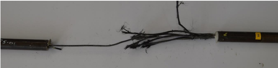
Figure 6.2-4 Failure of CFCC specimen at 347 °F (175 °C)
