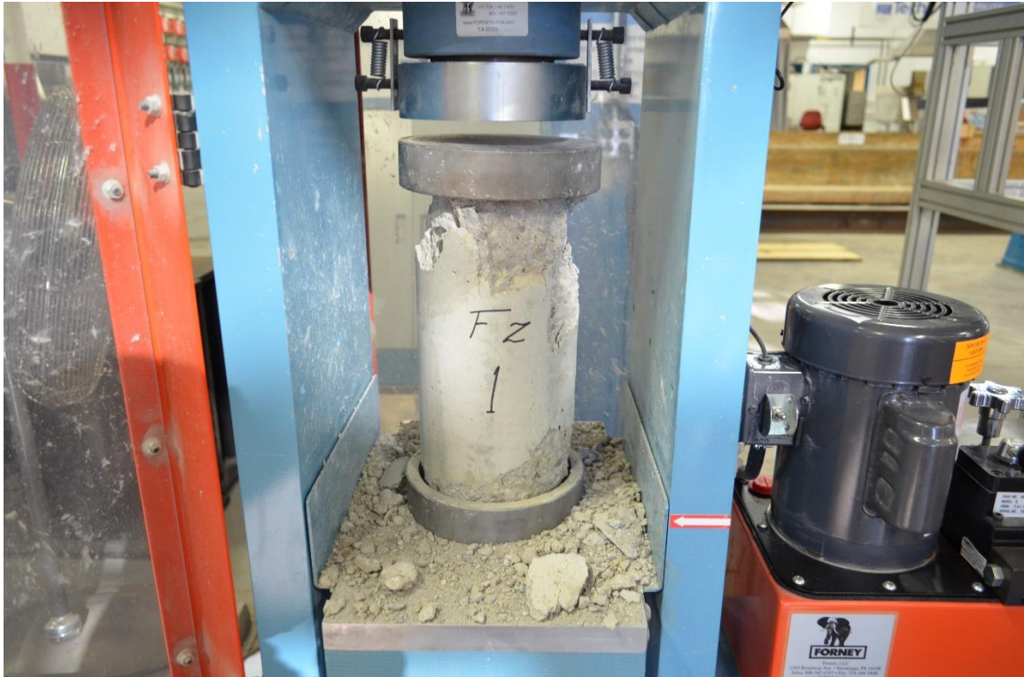
Figure 5.2-11 Testing and failure of cylinders after exposure to freeze-thaw cycles
