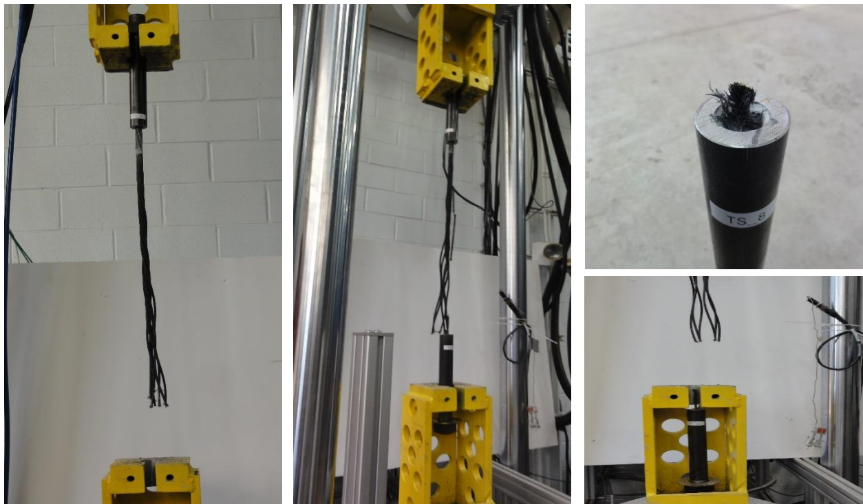
Figure 2.5-1 Typical failure mode of CFCC specimens with sleeve type anchorage
