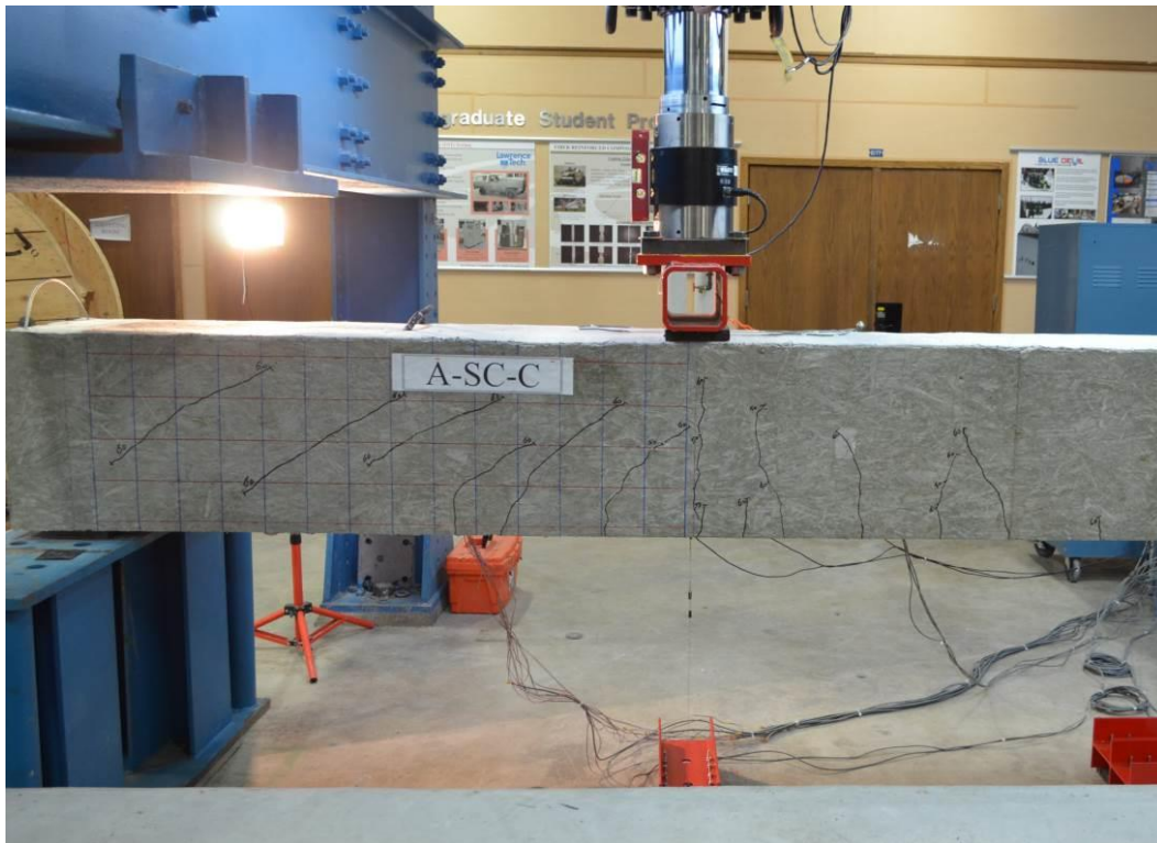
Figure 7.4-34 Crack pattern of beam S-C
