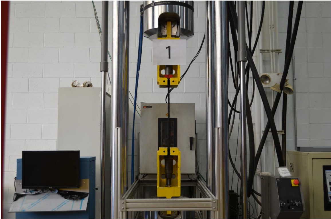
Figure 2.5-2 Uni-axial test setup for test specimens with wedge anchorage devices
