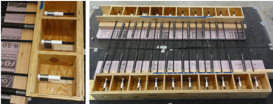
Figure 7.2-3 CFCC specimens in the formwork before pouring the concrete
