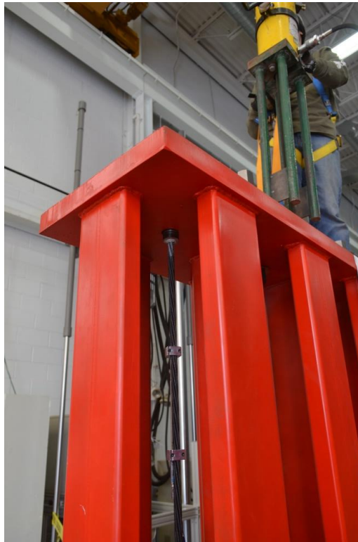
Figure 3.2-6 Strand-meter for strain evaluation in creep rupture specimens
