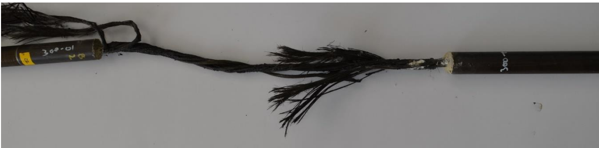
Figure 6.2-9 Failure of CFCC specimen at 572 °F (300 °C)
