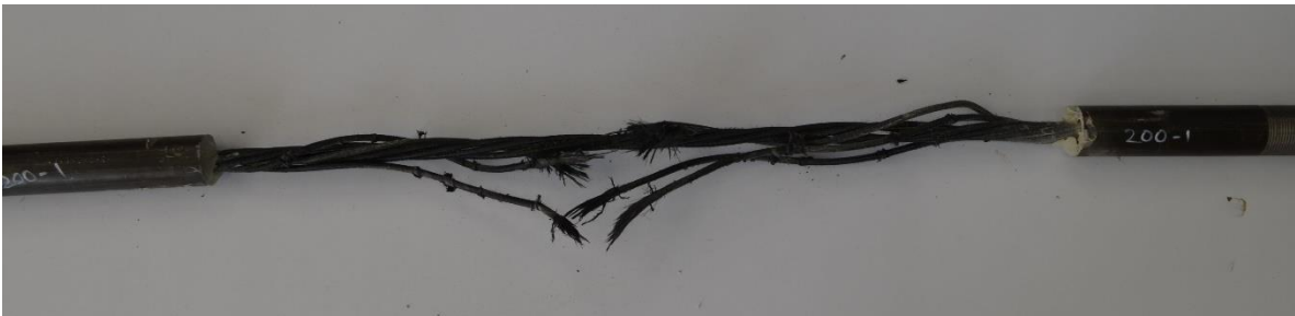
Figure 6.2-5 Failure of CFCC specimen at 392 °F (200 °C)
