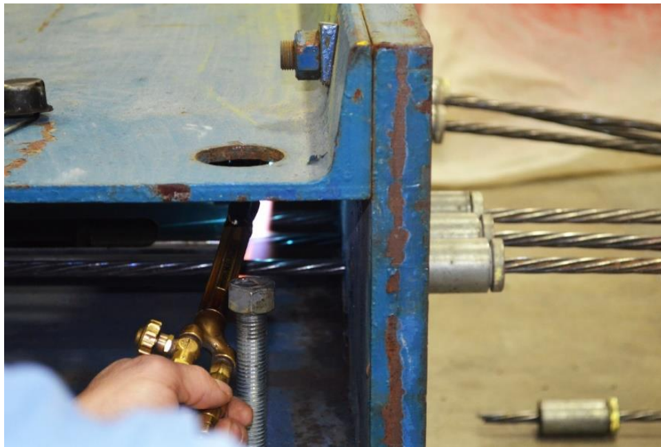
Figure 8.2-15 Release of steel strands at transfer
