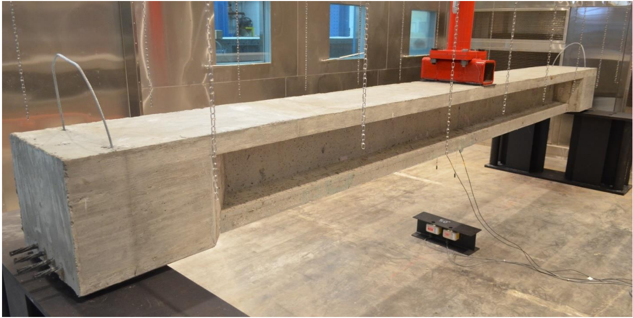
Figure 4.3-15 A decked bulb T beam under three-point loading in the environmental chamber
