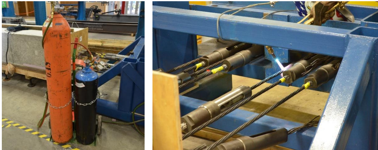
Figure 7.4-13 Releasing of prestressed strands
