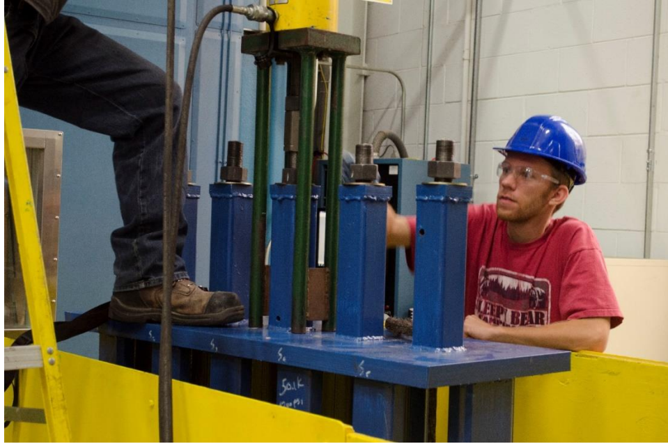
Figure 5.3-7 Releasing CFCC strands after freeze-thaw exposure
