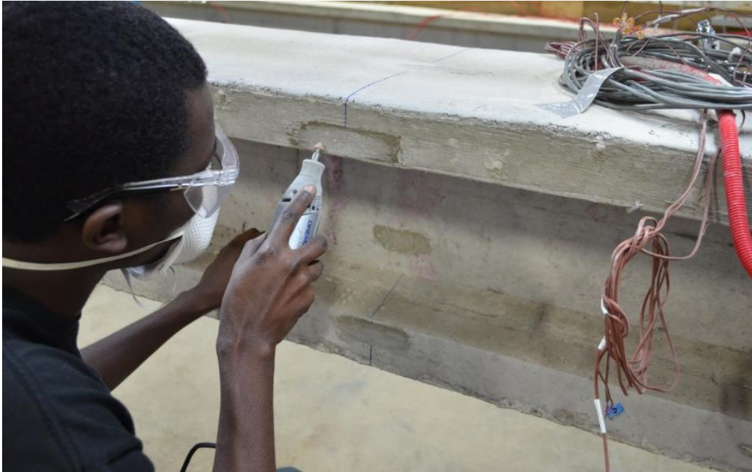
Figure 8.2-18 Smoothing the surface before installing strain gages
