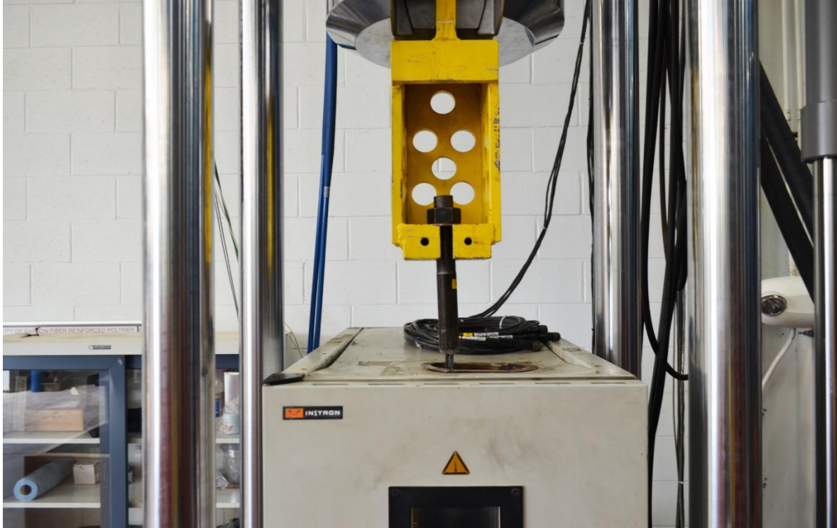
Figure 6.2-2 Anchorage device passing through a central opening in the heat chamber
