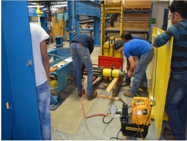
Figure 4.3-7 Applying prestressing force using a hydraulic pump
