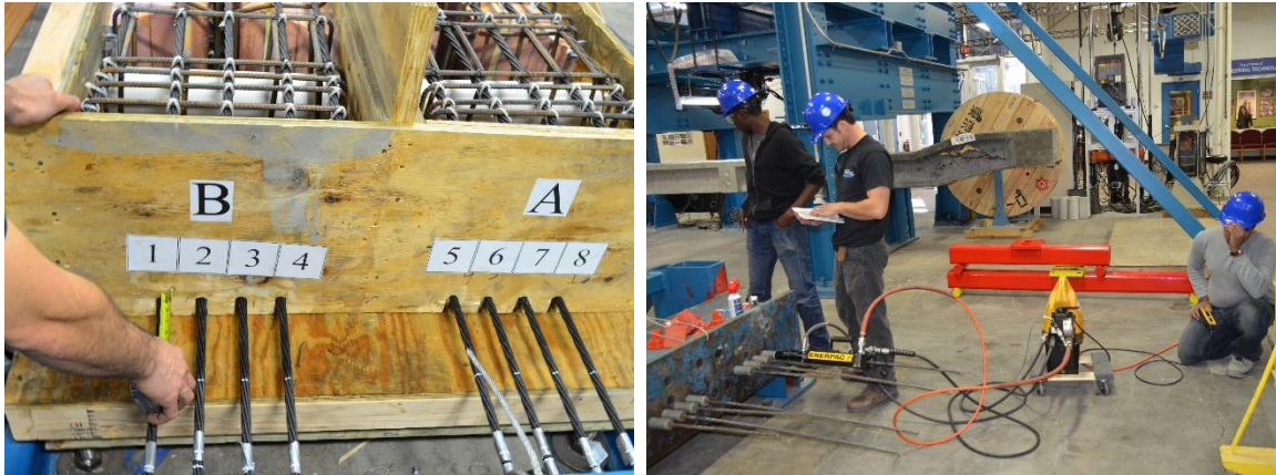
Figure 8.2-10 Layout and prestressing CFCC strands
