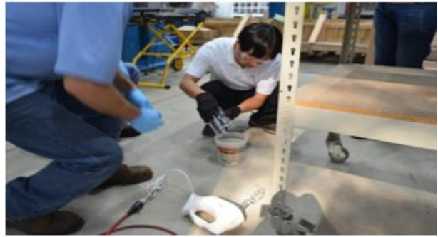
(b) Adding water and mixing HEM
