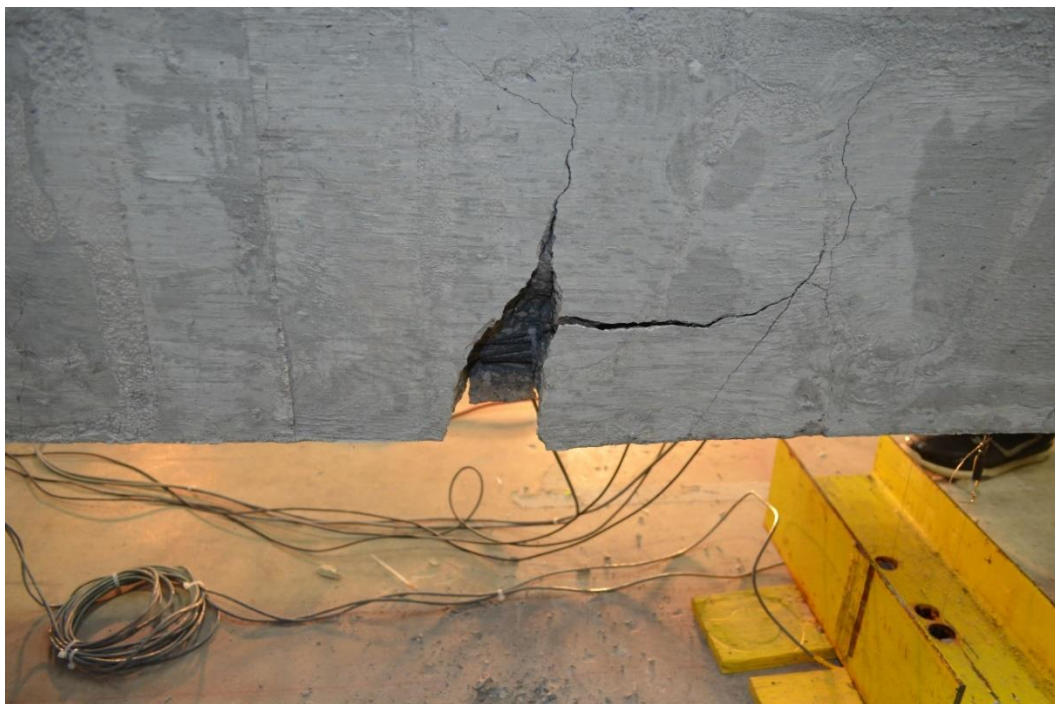
Figure 7.3-34 Cracking and failure of B3-0.6 at the end of the splice
