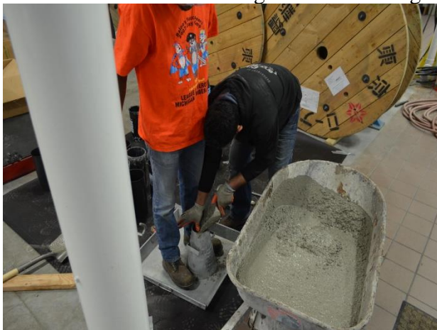
Figure 4.3-9 Slump test measuring 10 in. (254 mm)
