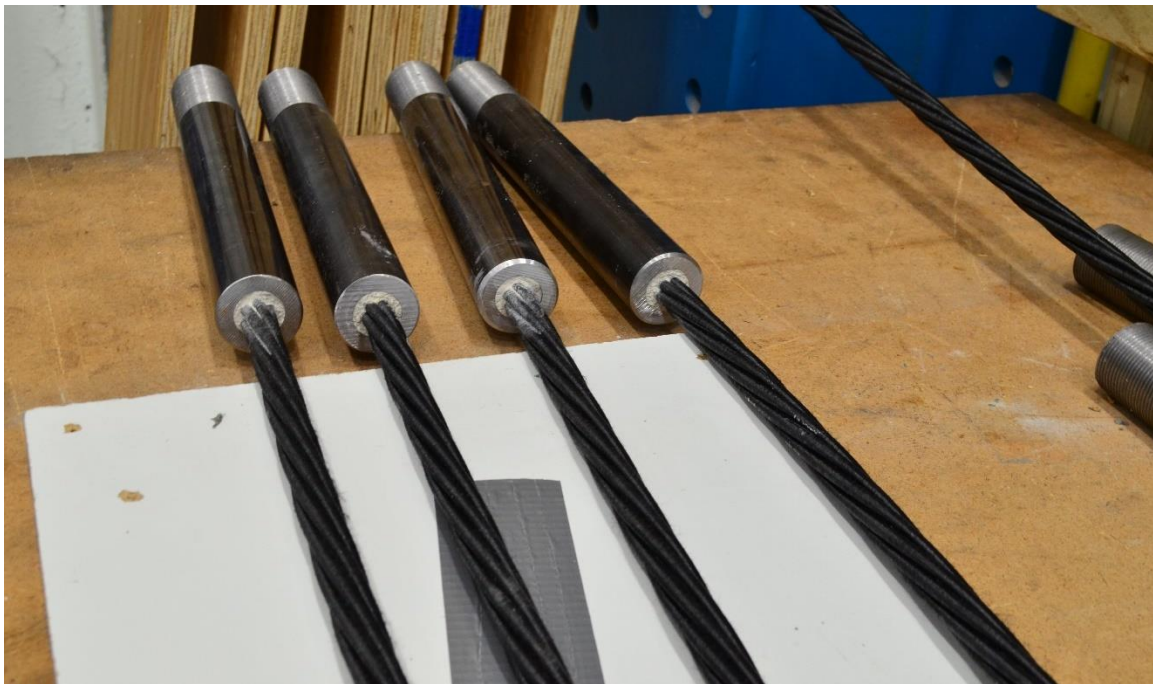
Figure 2.4-5 CFCC specimens with sleeve anchorage device after curing
