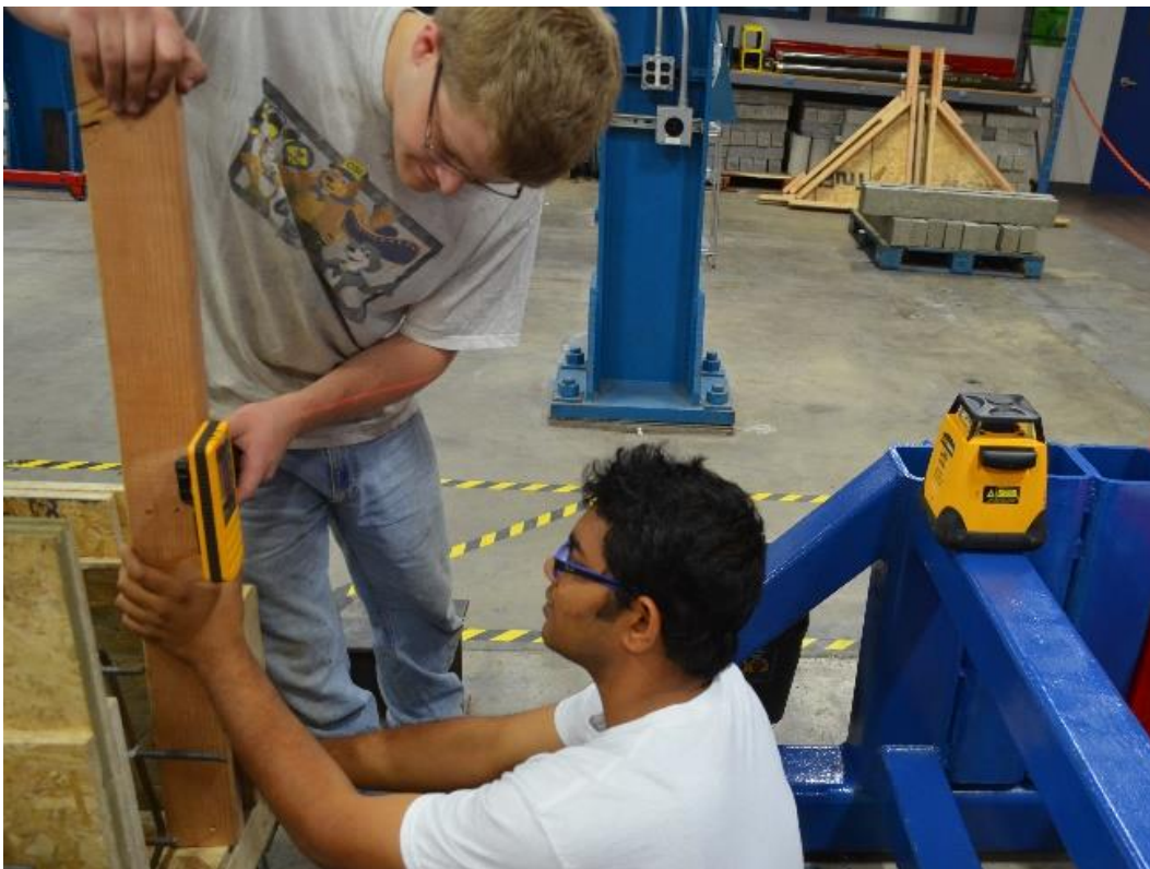
Figure 8.2-7 Leveling the platform using a laser level
