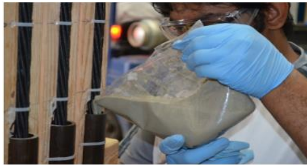
(c) Pouring HEM to the socket
