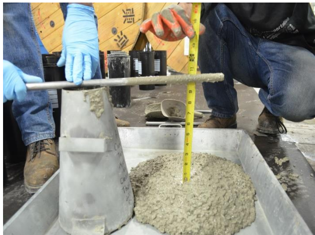
Figure 4.3-9 Slump test measuring 10 in. (254 mm)
