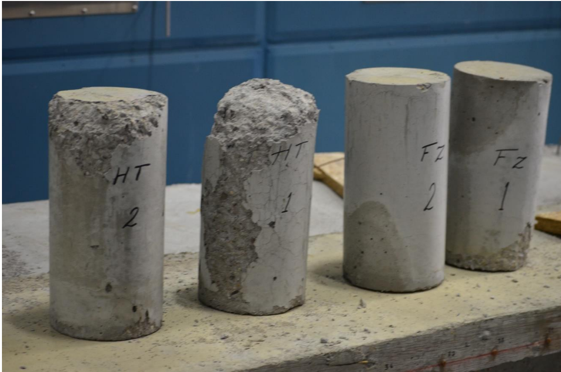
Figure 5.2-10 Concrete cylinders after exposure to 300 freeze-thaw cycles
