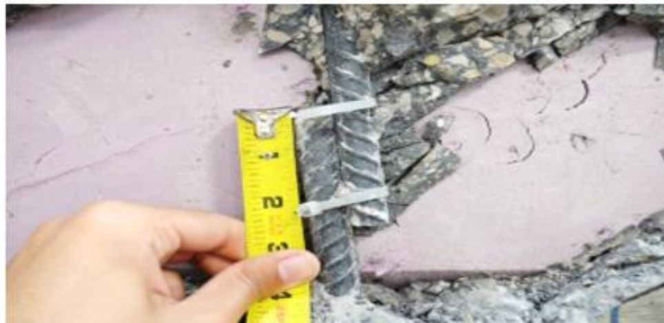
c) Slippage of the 4 in. (102 mm) spliced stirrups
