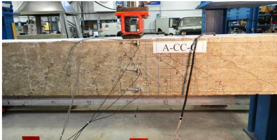
Figure 7.4-18 Crack pattern in beam C-C
