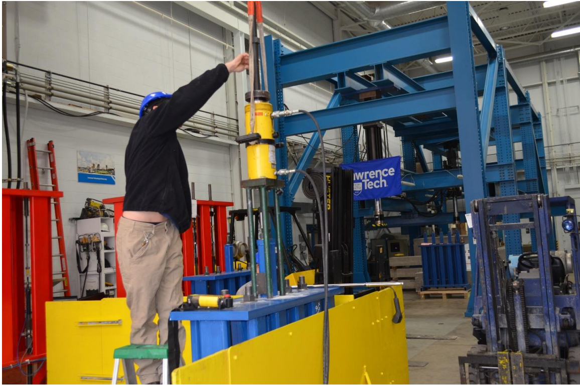
Figure 3.4-1 Stressing CFCC specimens for evaluation of long-term properties
