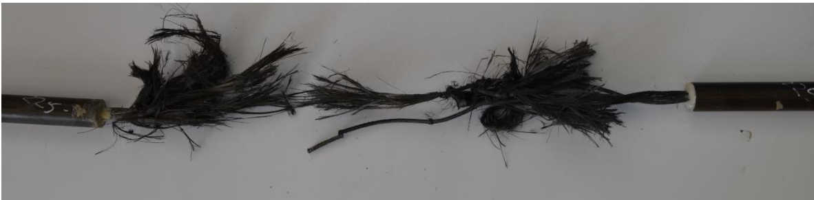
Figure 6.2-6 Failure of CFCC specimen at 437 °F (225 °C)
