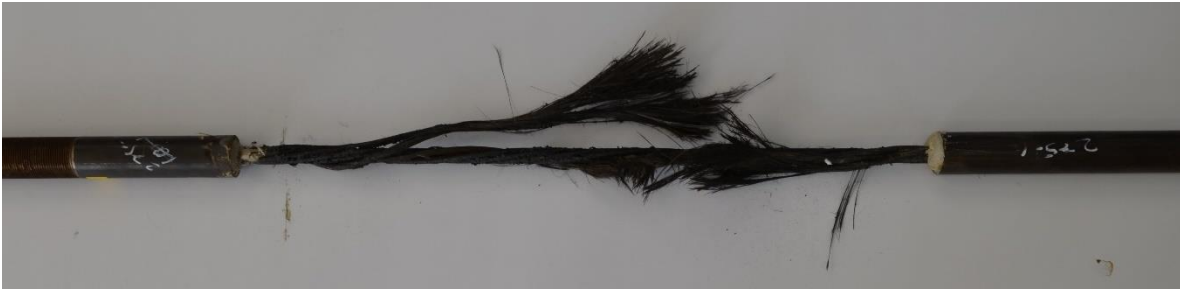
Figure 6.2-8 Failure of CFCC specimen at 527 °F (275 °C)
