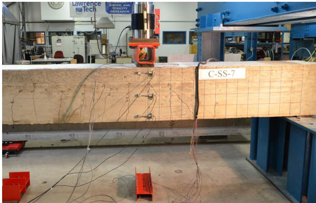
Figure 7.4-42 Crack pattern of beam S-7
