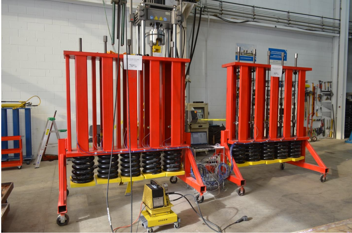
Figure 3.2-5 Two sets of creep rupture specimens prestressed to 70 % and 80 % of average tensile strength of CFCC
