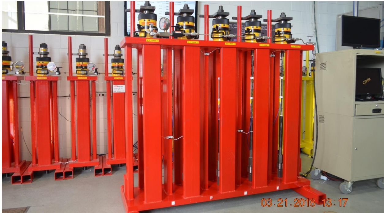
Figure 3.5-2 CFCC specimens under constant load to evaluate creep rupture strength
