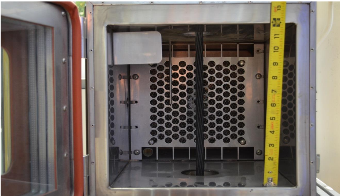
Figure 4.2-2 Heated length of CFCC strand inside the heat chamber
