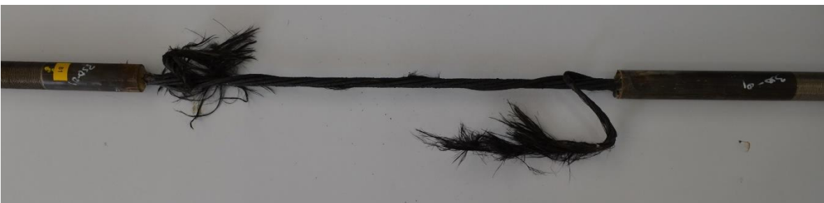
Figure 6.2-11 Failure of CFCC specimen at 662 °F (350 °C)
