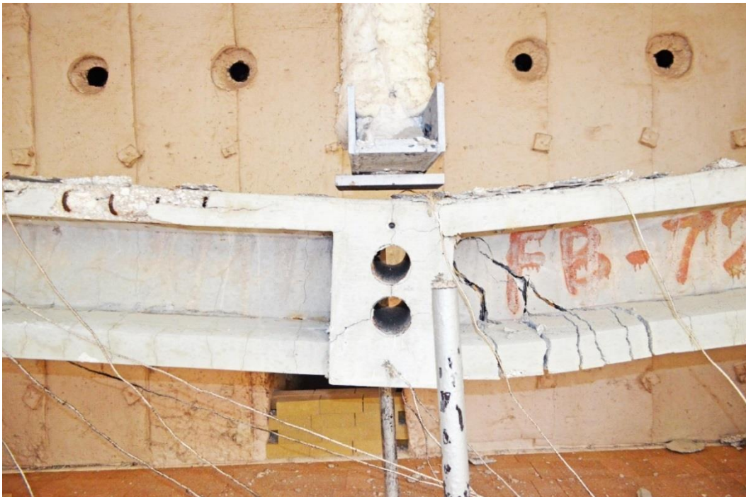
Figure 6.3-20 Close-up view of Beam C72-14-1 after failure
