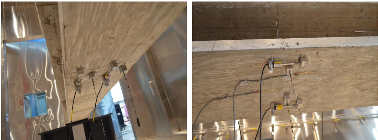
Figure 4.3-15 A decked bulb T beam under three-point loading in the environmental chamber
