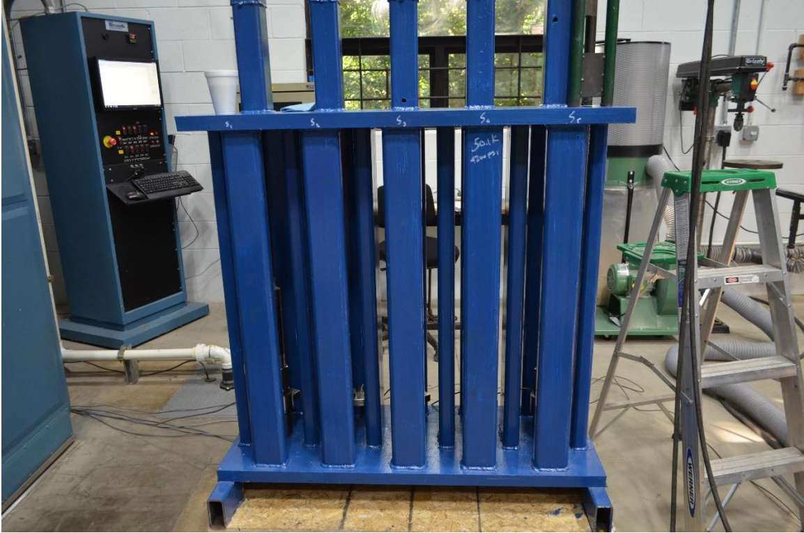
Figure 5.3-1 Steel frame to accommodate 4-ft-long CFCC specimens
