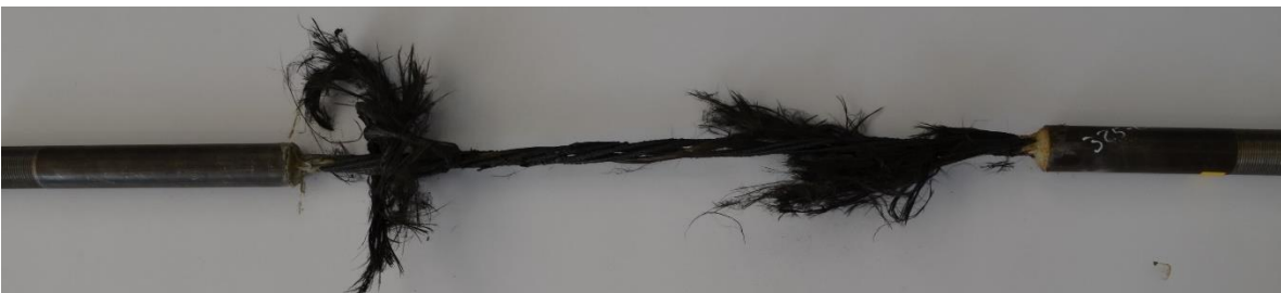
Figure 6.2-10 Failure of CFCC specimen at 617 °F (325 °C)
