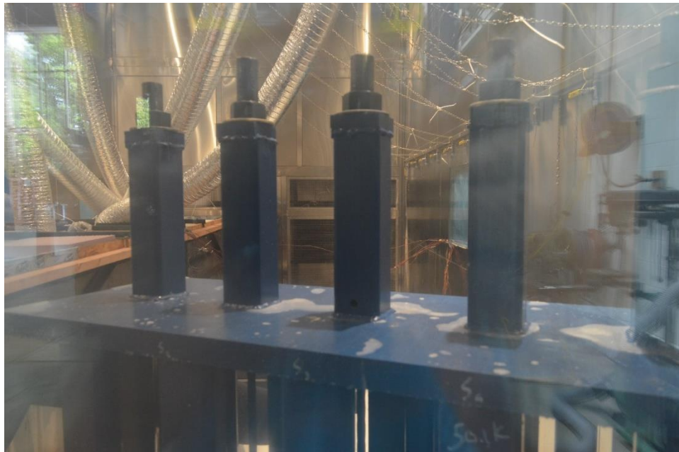
Figure 5.3-4 CFCC specimens during freeze-thaw testing
