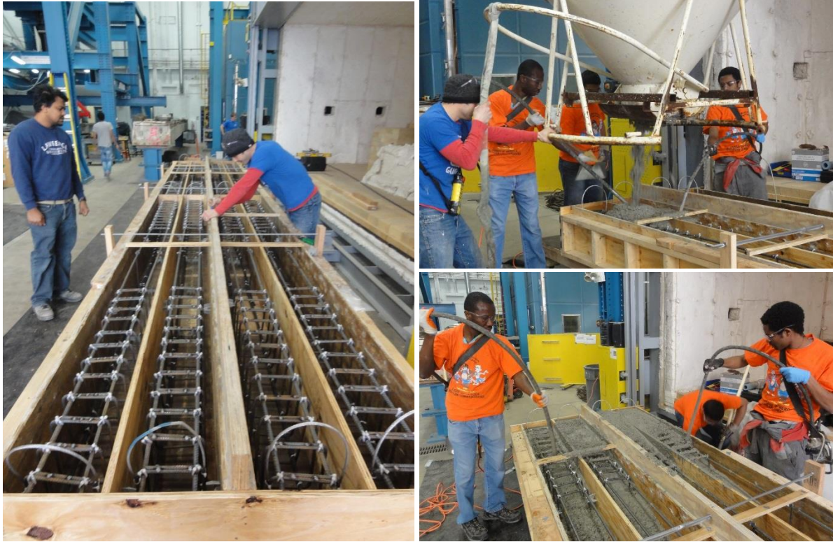
Figure 7.3-6 Casting the concrete in the test specimens
