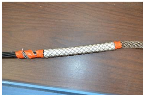
(b) Confinement with steel wire netting
