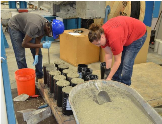
Figure 8.2-14 Placing and curing the concrete of the beams and cylinders
