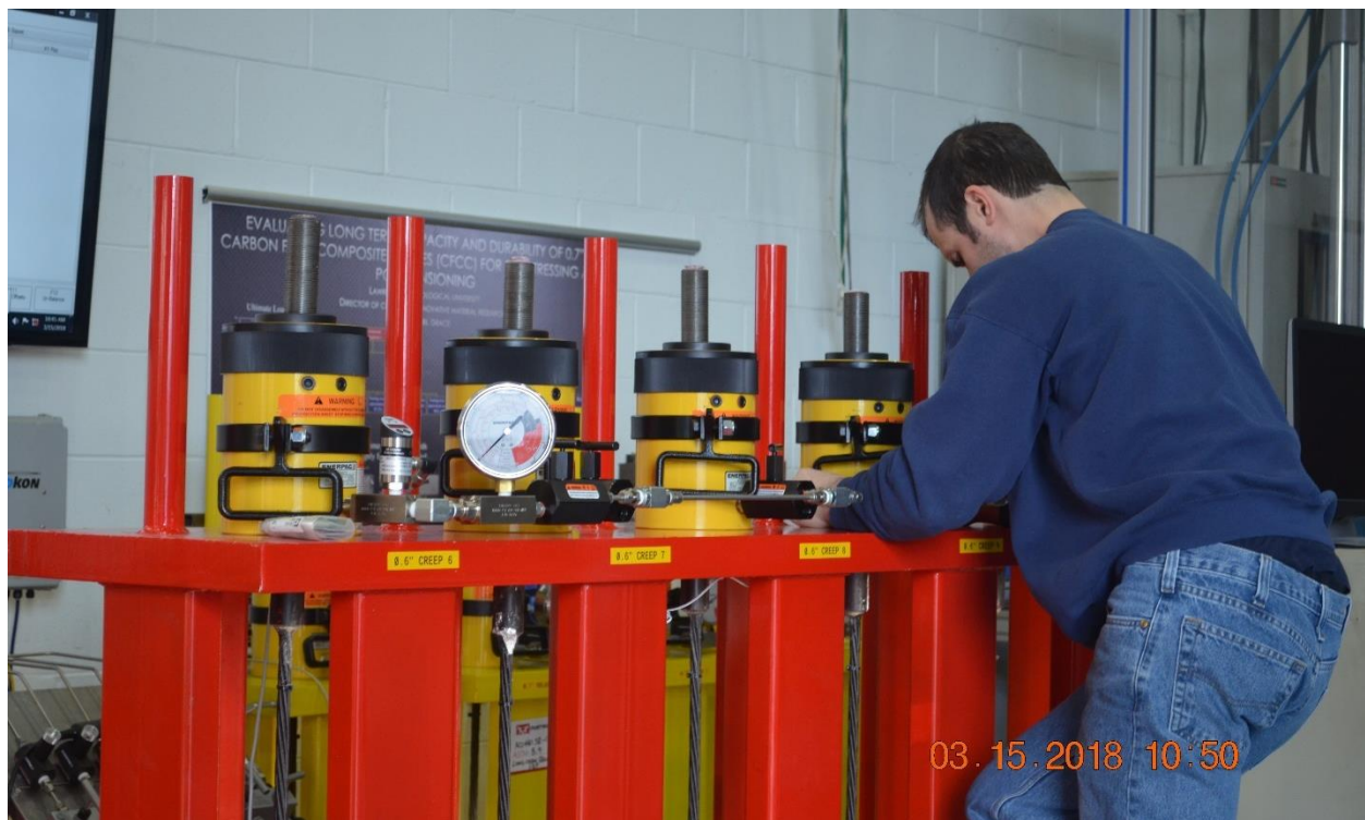
Figure 3.5-1. Closed-loop hydraulic system to maintain a constant force in creep test specimen
