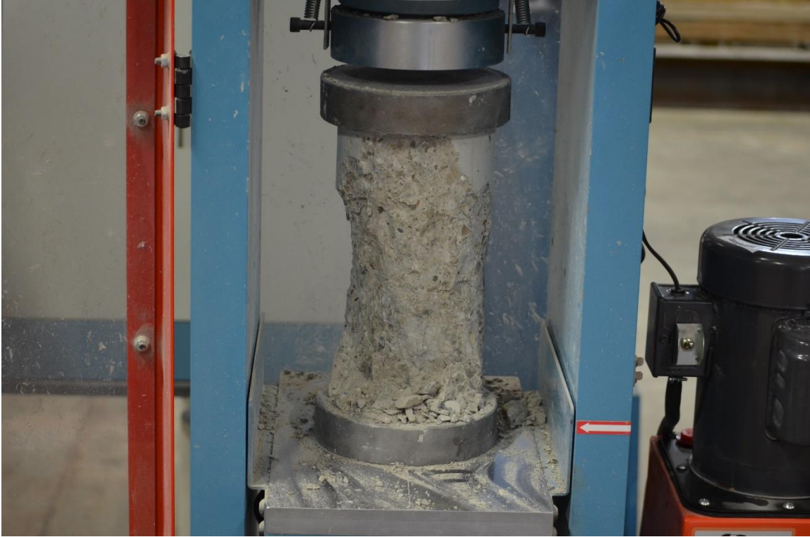
Figure 5.2-13 Testing and failure of control cylinders
