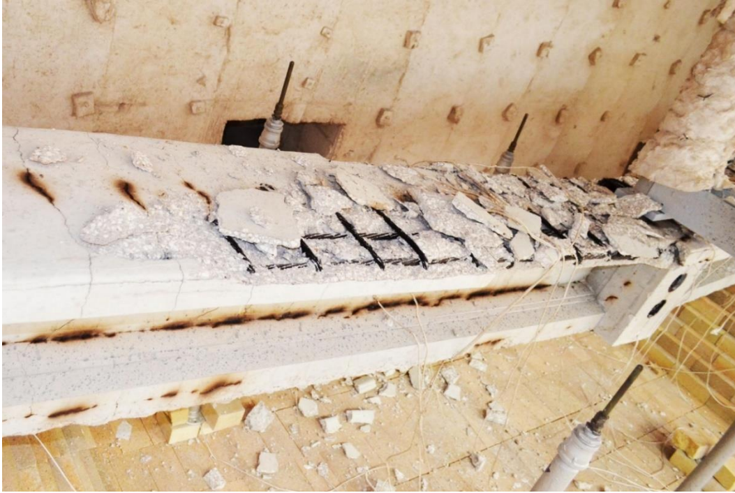
Figure 6.3-44 Concrete spalling of Beam C100-20-4 after fire
