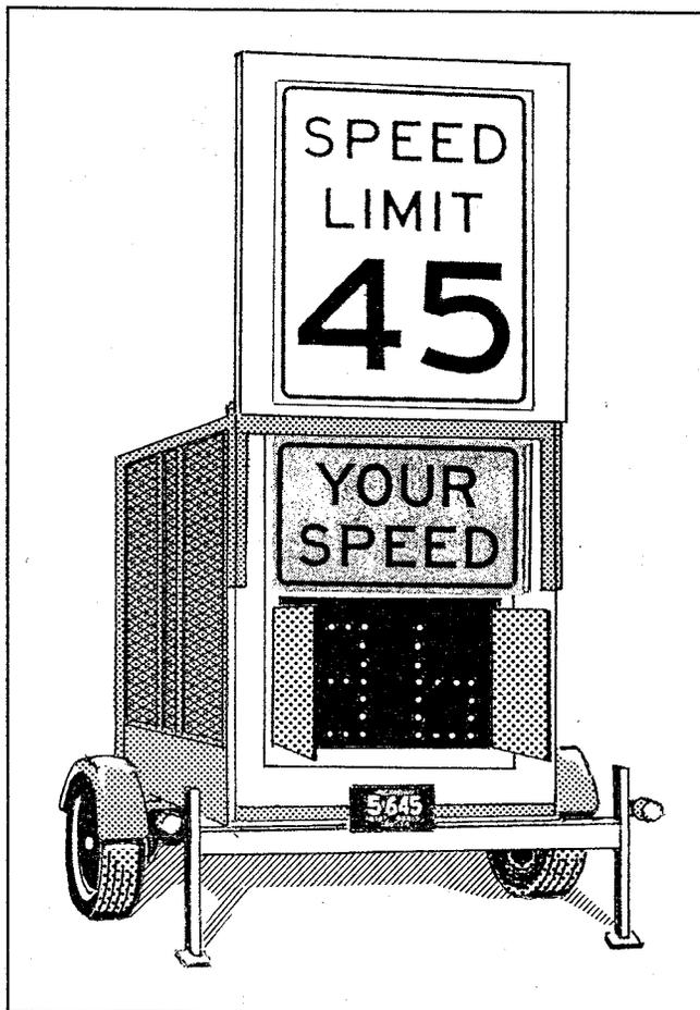
message. The static message consists of a standard roadway speed limit sign, with the appropriate posted speed limit for the area. Directly below that is a fixed panel that reads YOUR SPEED in black letters on an orange background. Below this panel is the changeable message portion of the sign. The sign trailer is parked at the side of the road and oriented such that the signs are clearly visible to approaching motorists.
