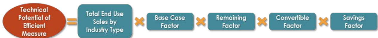
Equation 4-2: Core Equation for Commercial Sector Technical Potential
