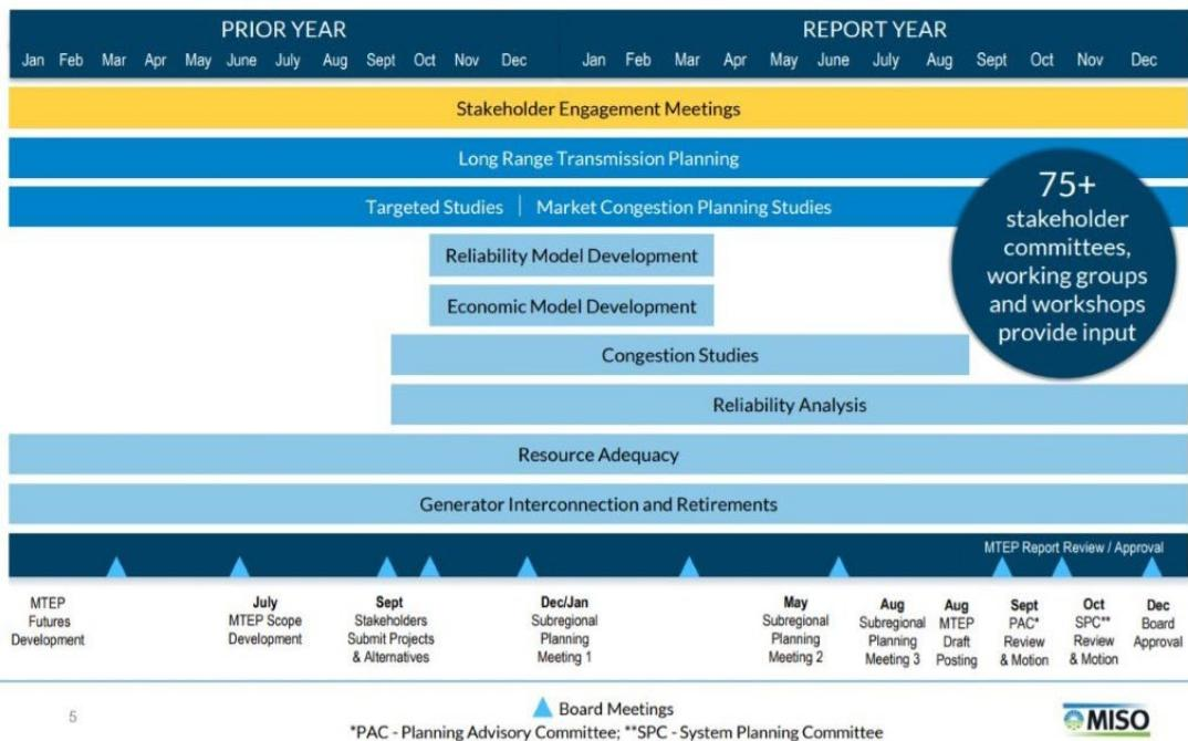
Figure 1 illustrates a typical MISO MTEP planning cycle. The RTOs conduct additional “top-down” planning to evaluate regional and interregional transmission drivers, including baseline reliability, economic efficiencies, long-range issues, and to enable public policy requirements. Outside of the formal expansion planning cycles, the RTOs may also conduct targeted studies to examine specific circumstances or policy studies to provide insight into emerging issues on the Bulk Electric System.
