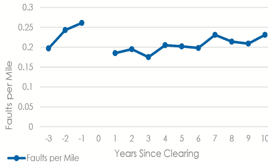
TREE-CAUSED FAULTS PER MILE BEFORE AND AFTER LINE CLEARING, 24.9-KV CIRCUITS
