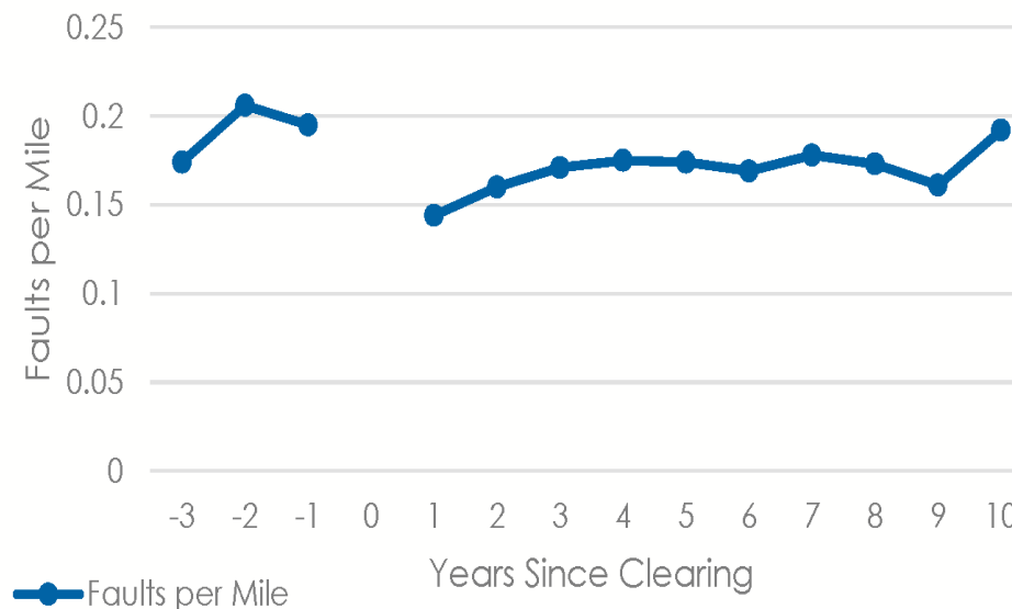
TREE-CAUSED FAULTS PER MILE BEFORE AND AFTER LINE CLEARING, 8.32-KV CIRCUITS
