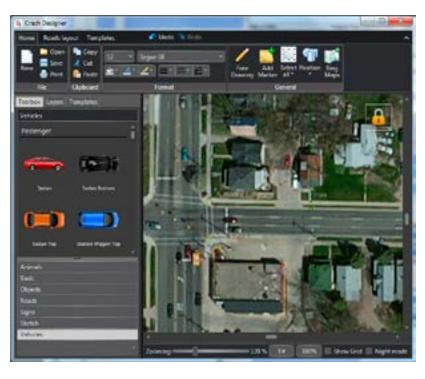
From this point, simply add the vehicles, pedestrians, road objects, etc. as you normally would. The iyeTek Crash Designer is a very robust diagramming tool that allows for total customization of the roadways and objects. Note: All objects can be sized to meet the scale of the roadway and placed in the proper lane.
