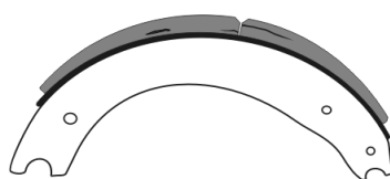
Cracks or voids that exceed 1/16" in width. Cracks that exceed 1-1/2" in length.
