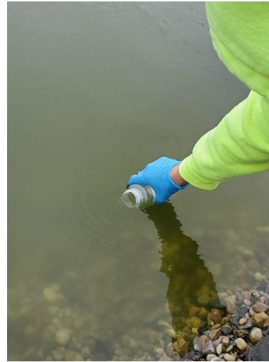
PHOTO 2. SUBJECT: Grab sample collection method at WWTP effluent, Lagoon 3. DATE: 21 September 2021. PHOTOGRAPHER: C.J.Lange.
