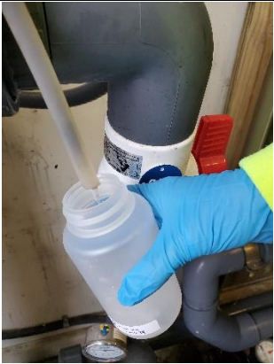
PHOTO 1. SUBJECT: Grab sample collection method at pre-treatment system influent sampling port, Building 1408. DATE: 21 September 2021. PHOTOGRAPHER: C.J.Lange.
