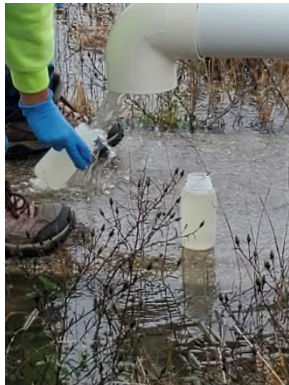
PHOTO 5. SUBJECT: Grab sample collection method at discharge from Pond 2 to rapid infiltration bed. DATE: 21 September 2021. PHOTOGRAPHER: C.J.Lange.
