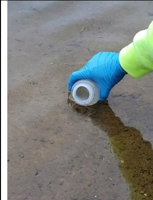
PHOTO 3. SUBJECT: Grab sample collection method at Pond 1 (sedimentation/separation tank) and Pond 2 (holding pond). DATE: 21 September 2021. PHOTOGRAPHER: C.J.Lange.
