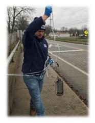
The weighted bottle sampler is typically constructed of a 1-liter Nalgene Tritan® bottle fixed inside a metal cage fitted with a weight below the bottle. This sampler is suspended vertically, which is ideal for sample collection at road or bridge crossings. The bottle is typically lowered to approximately 6-inches below the water surface. The sampler can also be fitted with a depth-integrating cap to allow the bottle to slowly fill while lowering the apparatus to the bottom of the water body.
