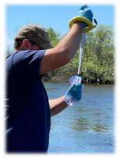
For surface water samples to be analyzed for PFAS using EPA SW-826 method 3512, the pipette method can be used to collect the sample. A pipette capable of collecting 10 milliliters (mL) of sample (e.g., the Gilson Pipetman Classic P10mL) should be used. The pipette tip should be constructed of PFAS-free material (e.g., polypropylene) and should be changed between samples. 5mL of sample should be dispensed into two laboratory-provided PFAS-free sample containers.
