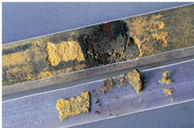
Photo 3: Geoprobe liner cut open to reveal soil sample. Samples are extracted using clean utensils or gloves from core into appropriate sample containers.
