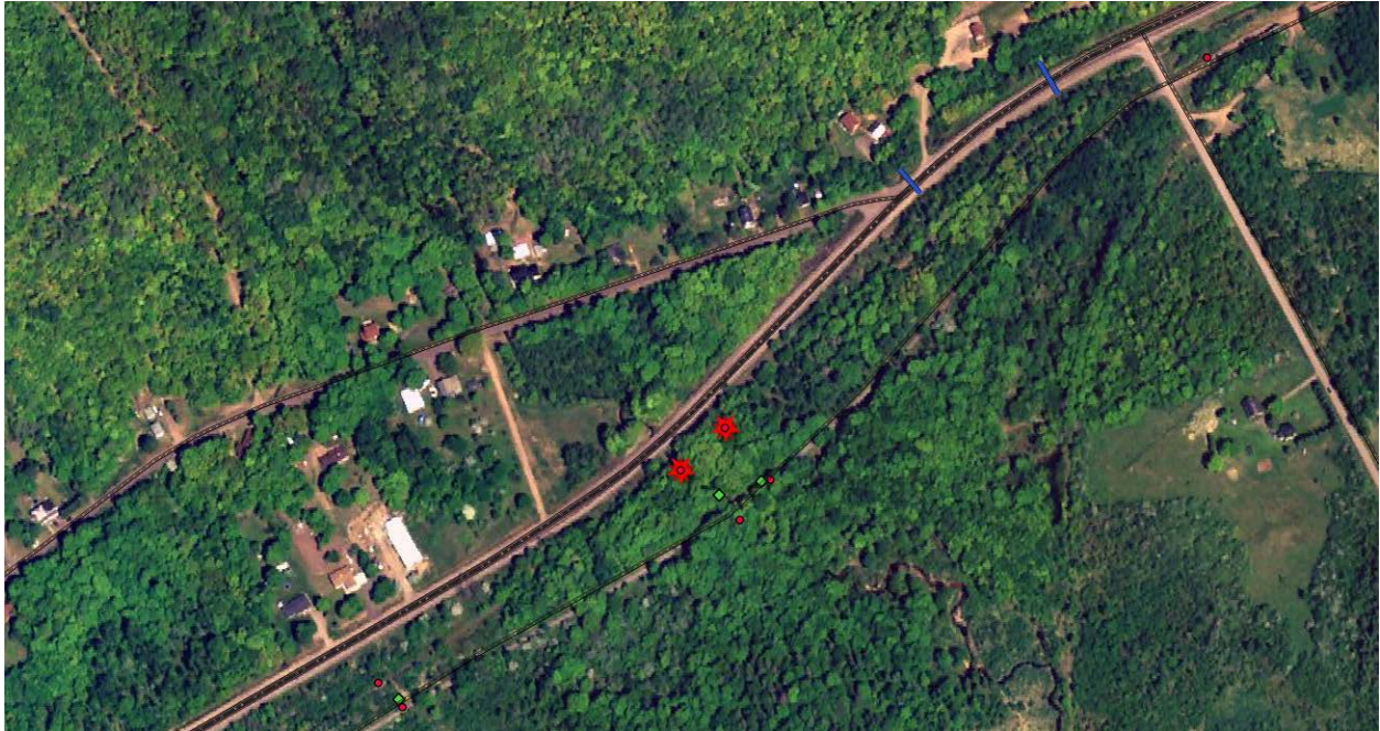
Figure 8: Potential new MDOT culverts shown as red stars. Existing MDOT culverts shown as dark blue lines, DNR bridges and culverts shown as green diamonds and other stream crossing surveys shown as red circles.
