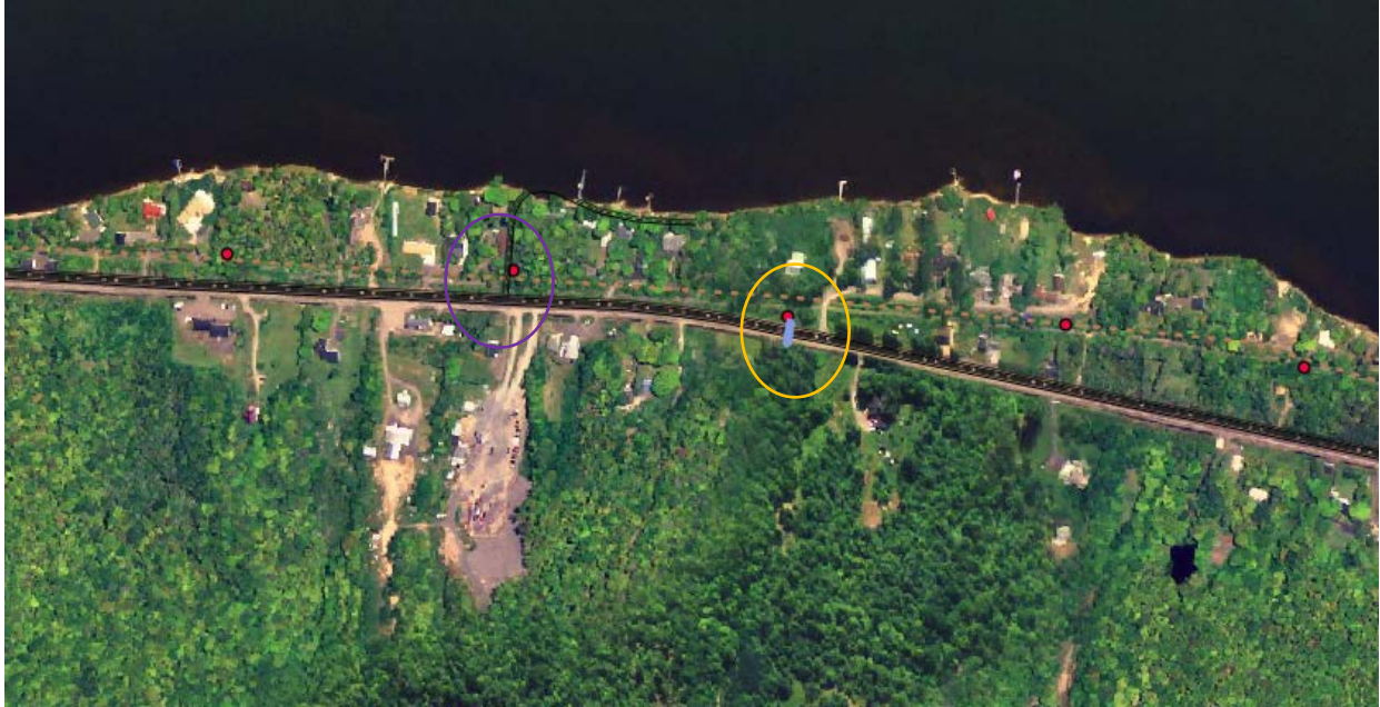
Figure 1: DNR Trail located adjacent to MDOT owned highway and crossing local roads. MDOT culverts shown in blue, DNR Stream crossings (culverts) shown in red.
