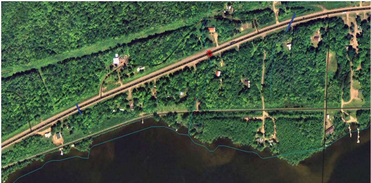
Figure 6: Potential new MDOT culvert shown as red star. Known MDOT culverts shown as dark blue lines, other stream crossing surveys shown as red circles.
