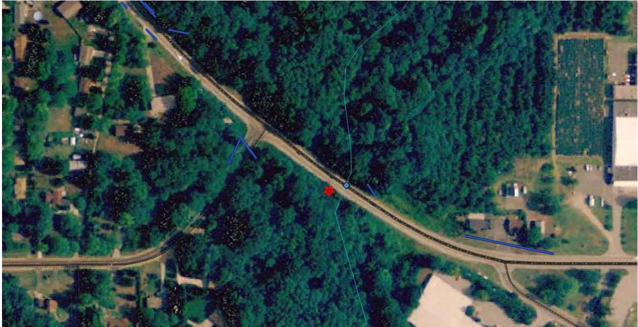
Figure 5: False positive new MDOT culvert shown by red star icon. MDOT bridge shown as blue diamond, MDOT culverts shown as dark blue lines.
