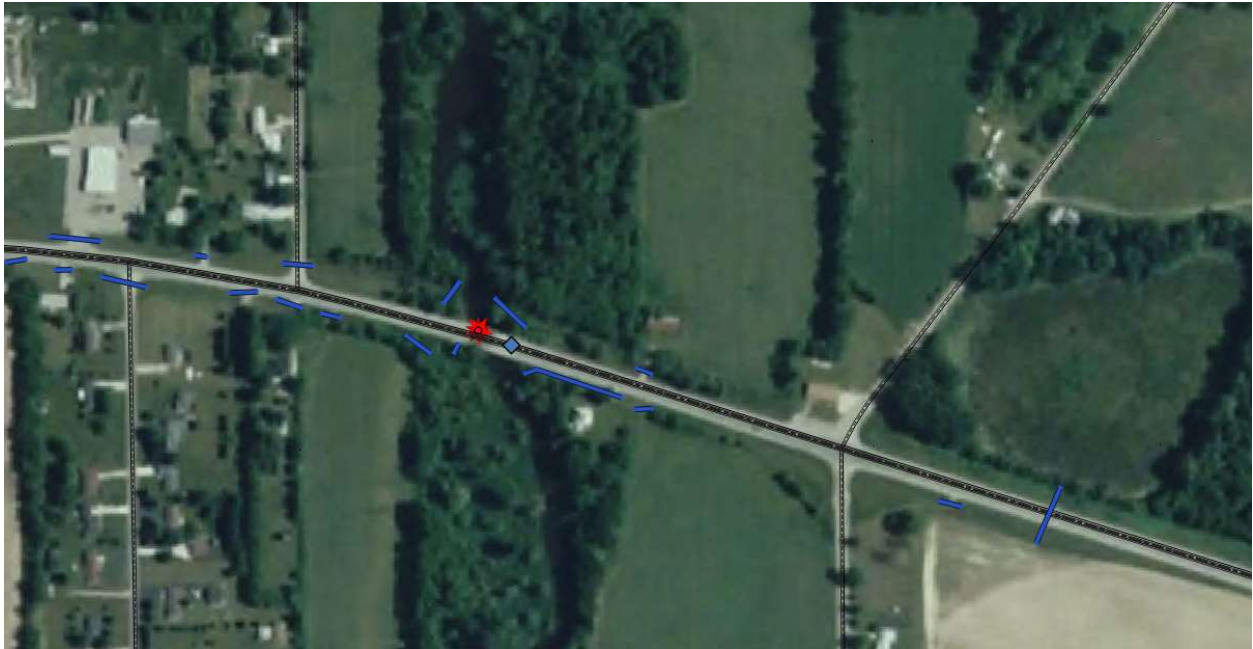
Figure 3: False positive new MDOT culvert shown by red star icon. MDOT bridge shown as blue diamond, MDOT culverts shown as dark blue lines
