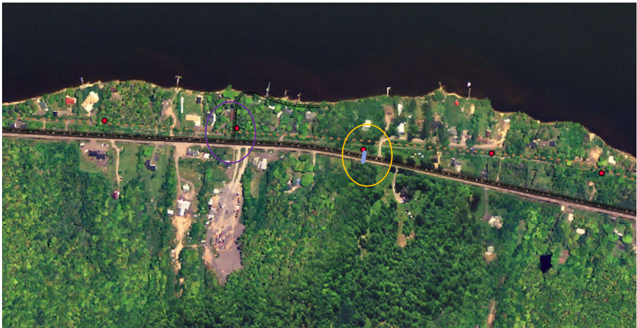
Figure 1: DNR Trail located adjacent to MDOT owned highway and crossing local roads. MDOT culverts shown in blue, DNR Stream crossings (culverts) shown in in red.
