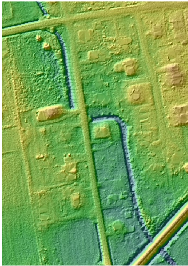
Figure 4: The 2 ft DEM contains some artifacts such as the lines visible in the bare earth that require correcting before hydro-enforcement can be undertaken.
