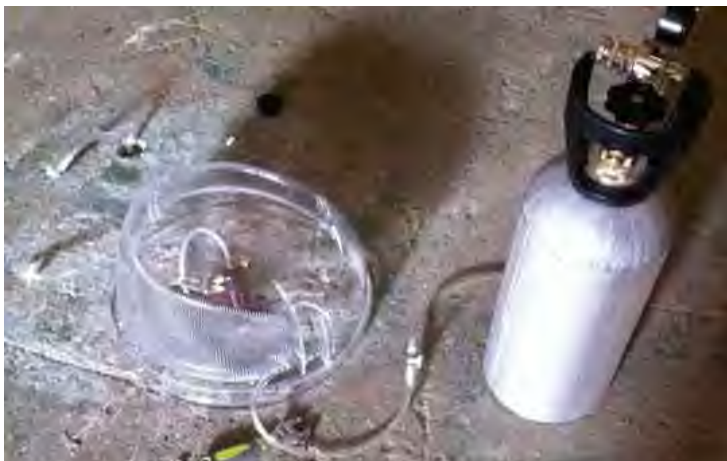
Figure 1. Sampling shroud being pressurized with helium.
