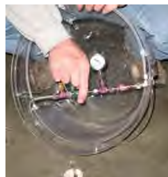
Figure 6. Connect regulator assembly to shroud.
