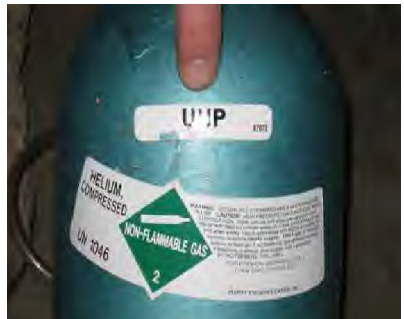
Figure 2. Use Ultra High Pure (UHP) grade helium to avoid background contaminants.
