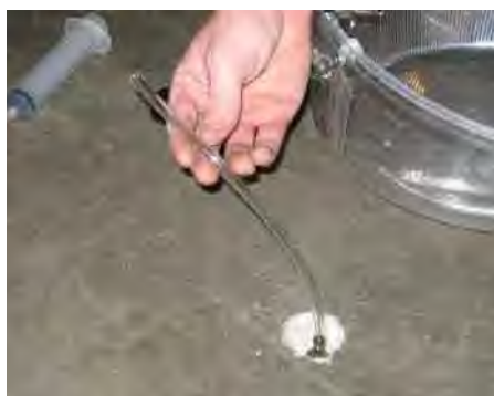
Figure 4. Connect sampling line to point.
