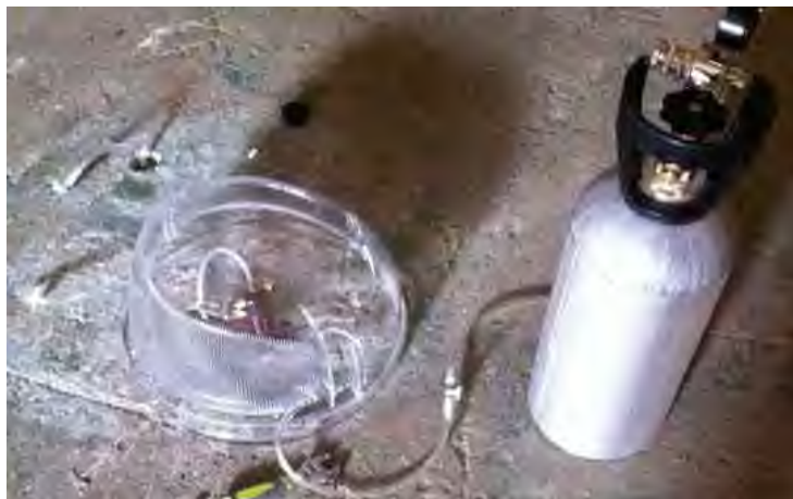
Figure 1. Sampling shroud being pressurized with helium.
