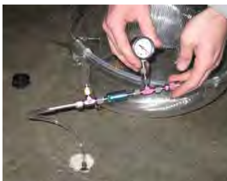
Figure 5. Connect regulator to sampling line.
