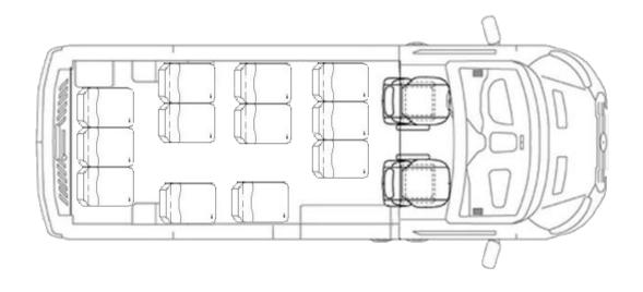
Class IV – 148" Wheelbase, Dual Rear Wheels, Fourteen Passenger w/Driver
