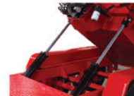
Dump System - Pivot Point & V-Body
