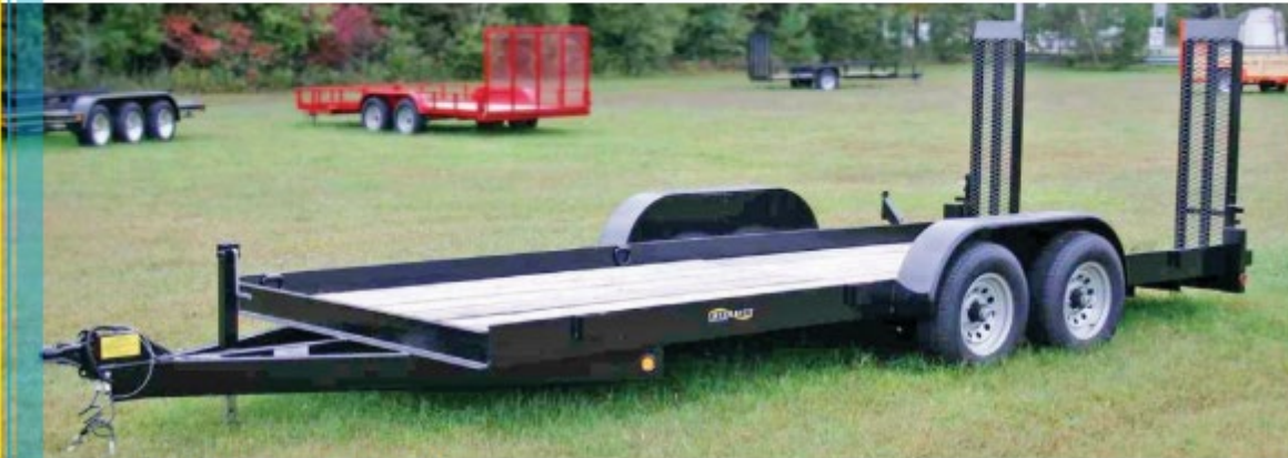
80' x 18' Tractor/Skid Steer Trailer, 9,900 GVW
