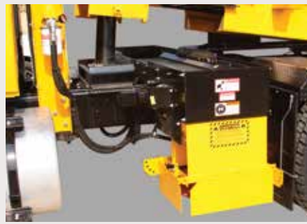
Front Cross Conveyor with Two Ply High-Temp Rubber Belting and Front Mounted Spinner
