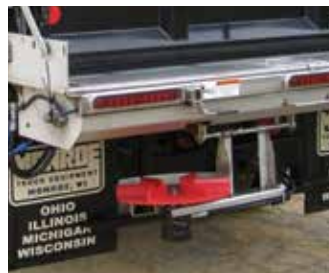
Self Leveling Spinner without Stabilizer Rod
