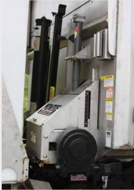
25:1 Drive System & Screw Adjustable Gate
