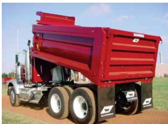
Figure: Shown with optional metal boards, tarp system, lights in rear crossmember, and tow package.
