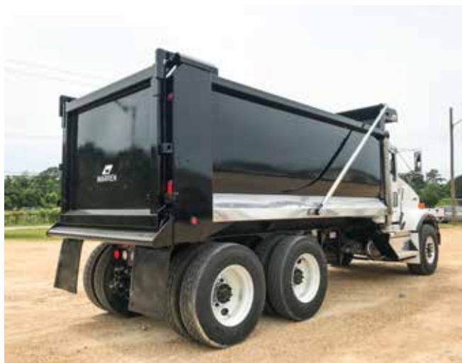
Figure: Shown with optional High lift Tailgate, aluminum fender covers, TARP system & D/S WAR Steps .
