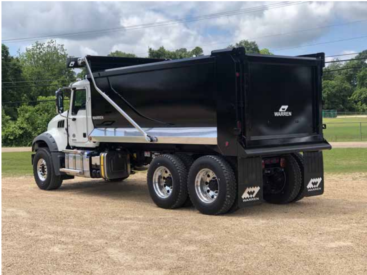
Figure: Shown with optional High lift Tailgate, aluminum fender covers & TARP system.
