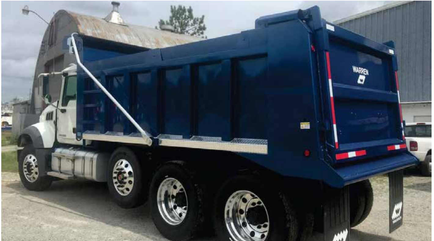
Figure: Shown with vertical side braces, optional high lift tailgate, and upgraded metallic paint
