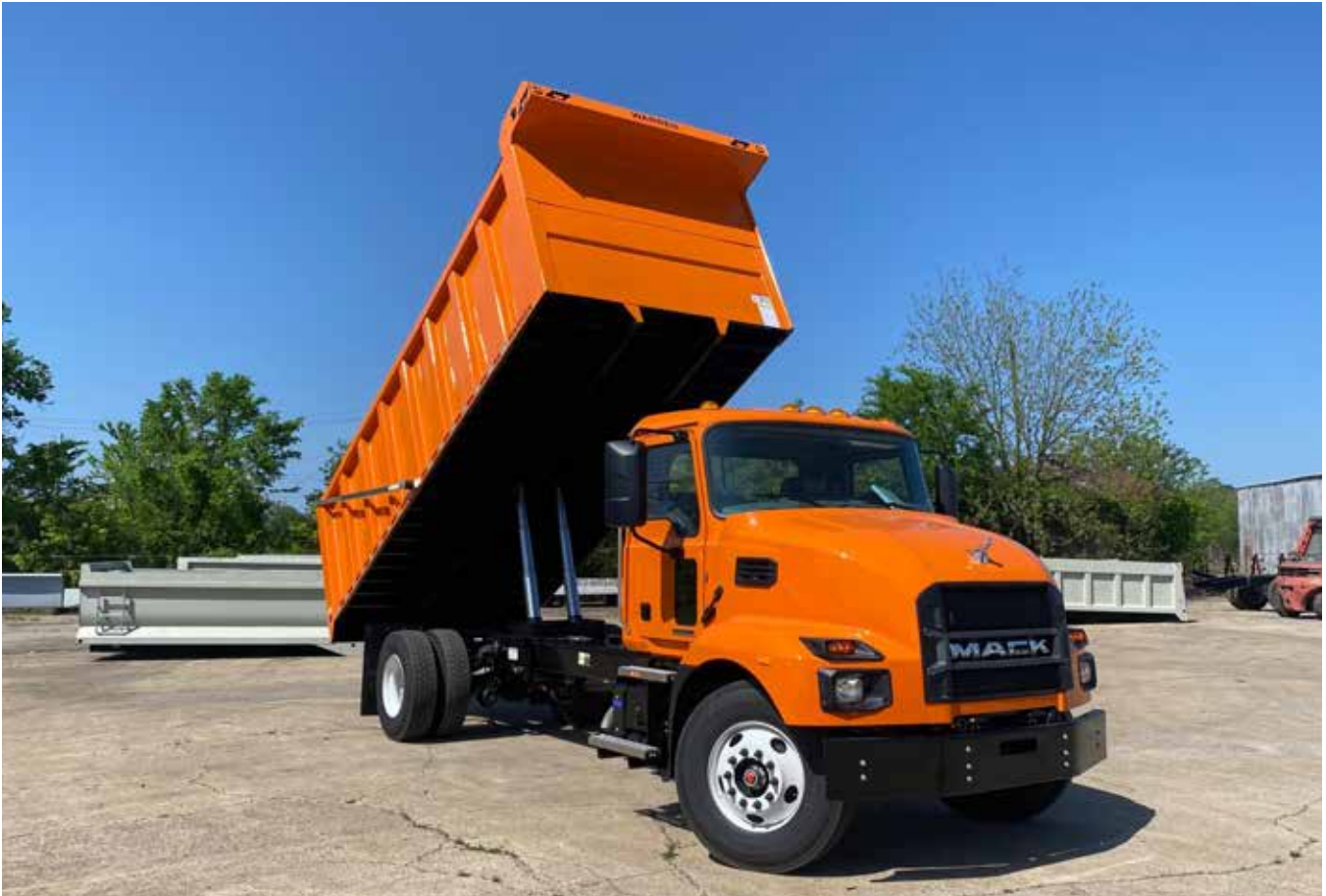
Figure: U-10 with underbody hoist and optional Cabshield, TARP system & Custom Paint.
