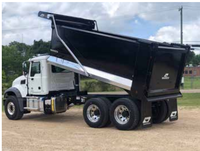
Figure: Shown with optional High lift Tailgate, aluminum fender covers, TARP system & D/S WAR Steps .
