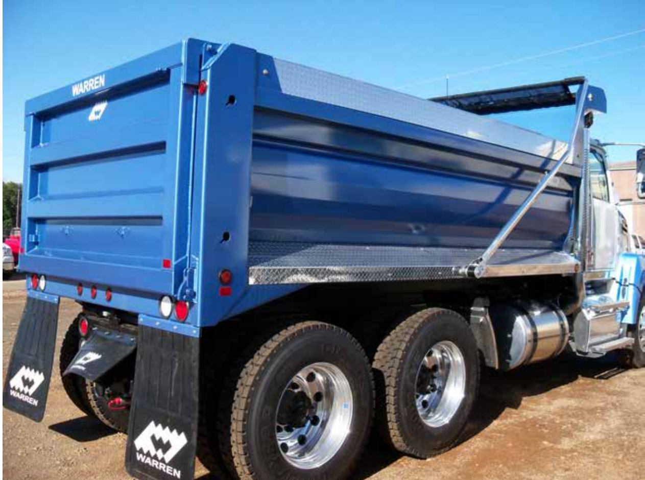
Figure: Shown with optional metal boards w/ aluminum covers, aluminum fender covers, and TARP.
