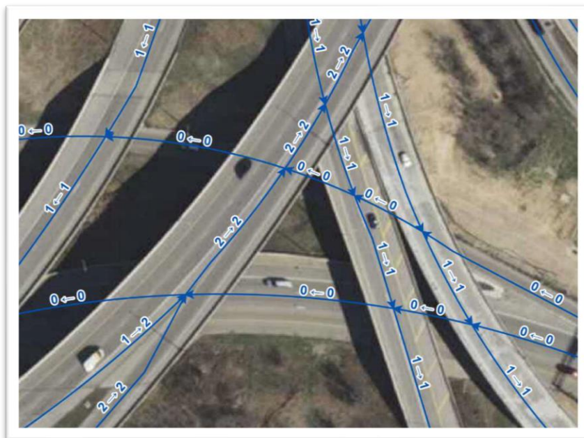
Figure 5-5 Road Centerline Segments with Elevation Attribution
