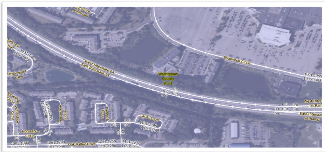
Figure 5-2 Road Centerlines digitization with direction of travel
