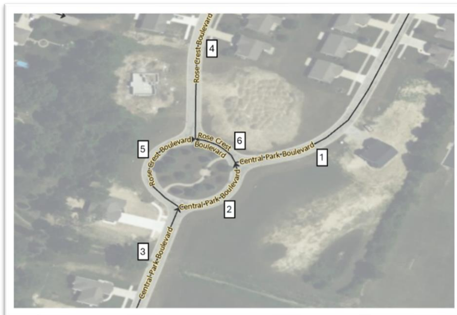
Figure 5-12 Roundabout with Road Ending at the Roundabout
