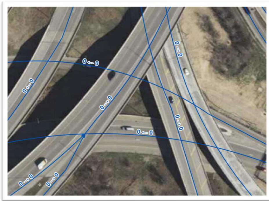
Figure 5-4 Road Centerlines Without Elevation Attribution
