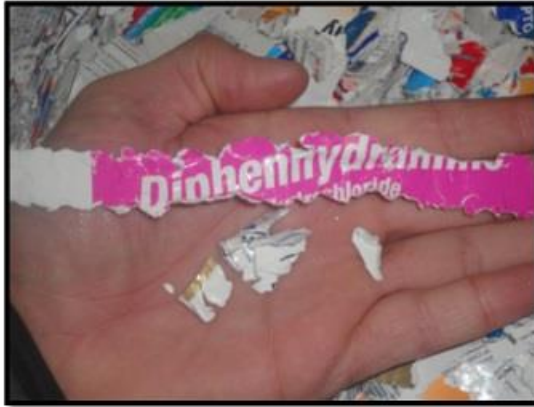
strip cut shred compared to grinder shred
