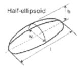
Half-ellipsoid: If the pile is more the shape of a half-ellipsoid, like the one shown here, then multiply Pi (3.14) by the length by the width by the height and divide by 6.
