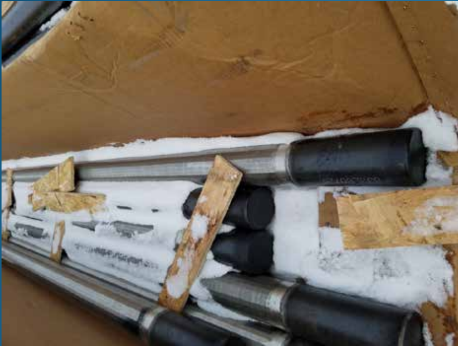
MPE Well w/Sump
