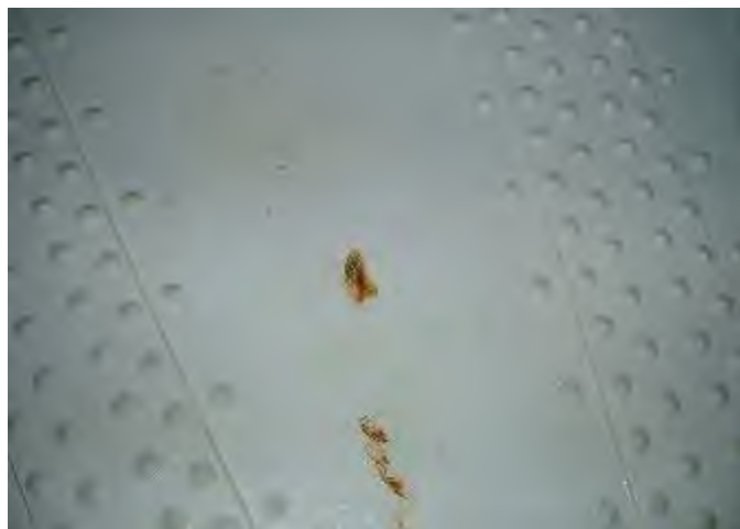
(33) Coating break and rusting on upper bowl.
