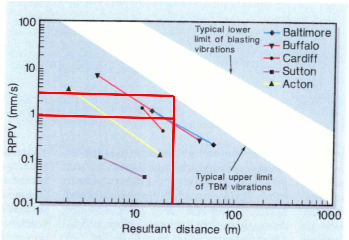
Figure 1: TBM Vibration Attenuation Data from Prior Projects (Flannagan 1993)
