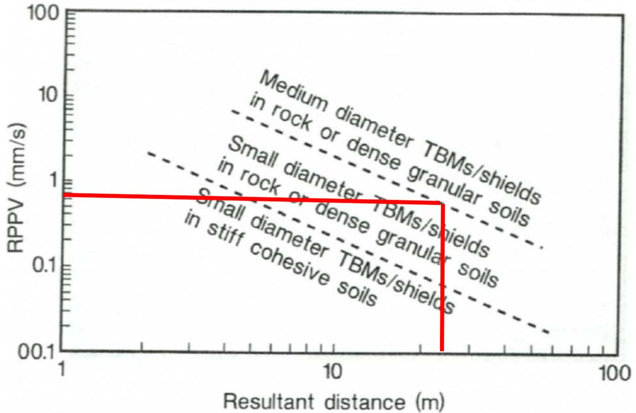
Figure 2: Vibrations from Small to Medium sized TBMs (Flannagan 1993)
