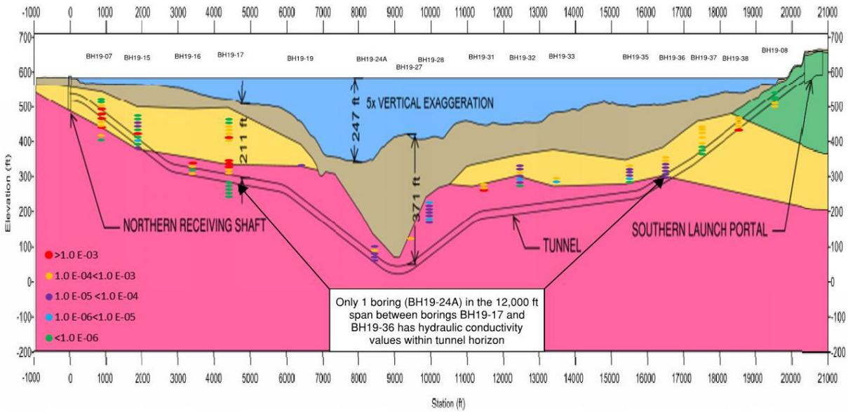
**Figure 4: Hydraulic Conductivity along proposed alignment**
