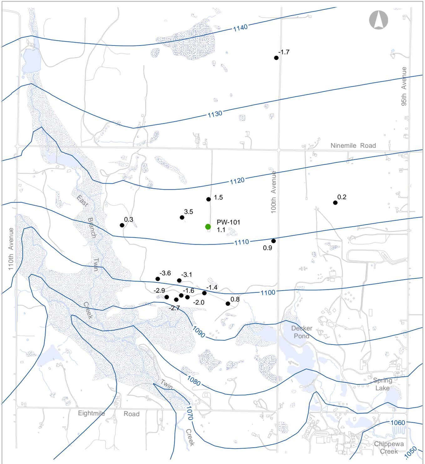
— 1110 — Contour of Water Levels in Model Layer 3 (feet, MSL)
