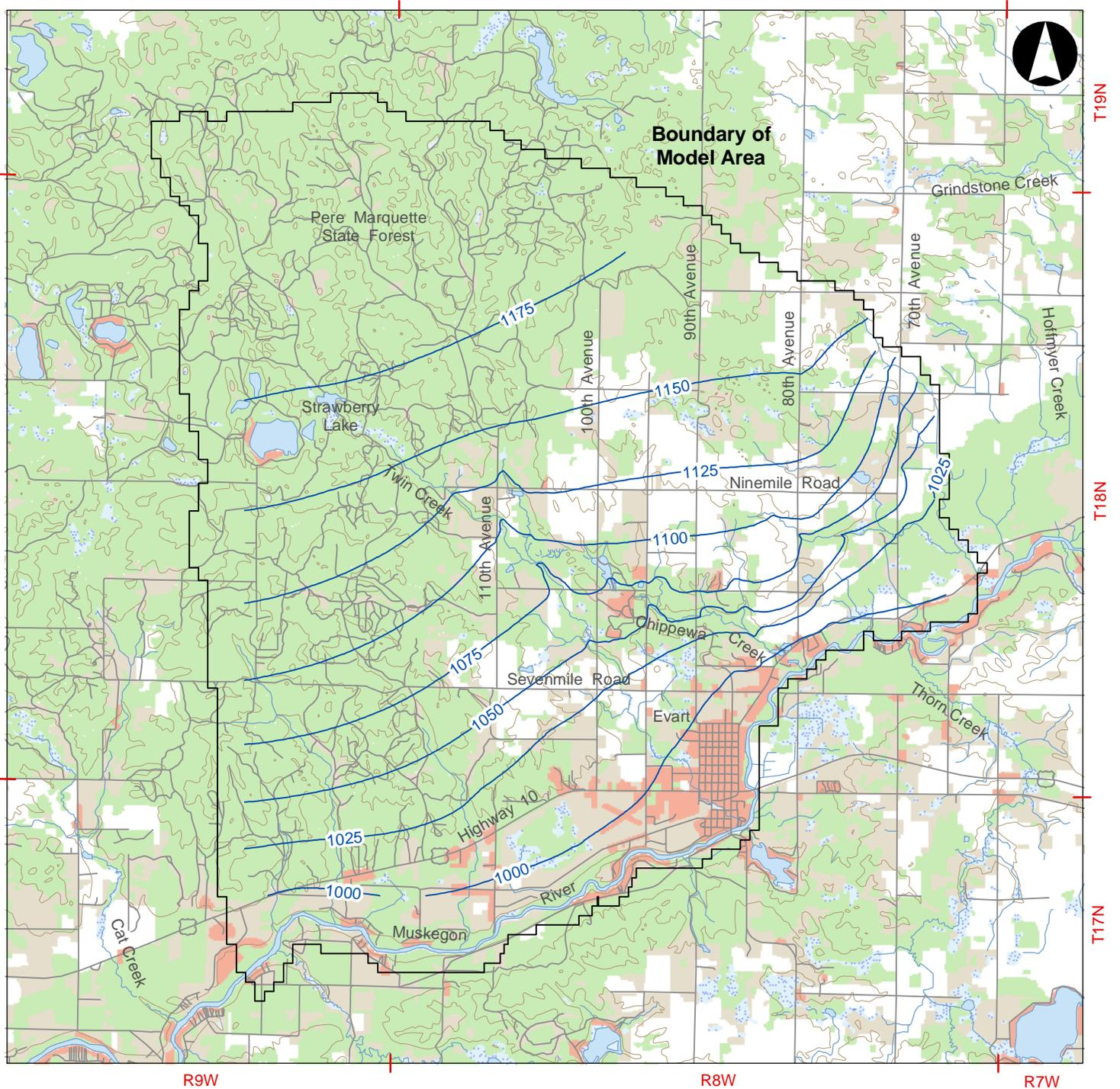
— 1000 — Contour of elevation of water-table surface (feet, MSL)
