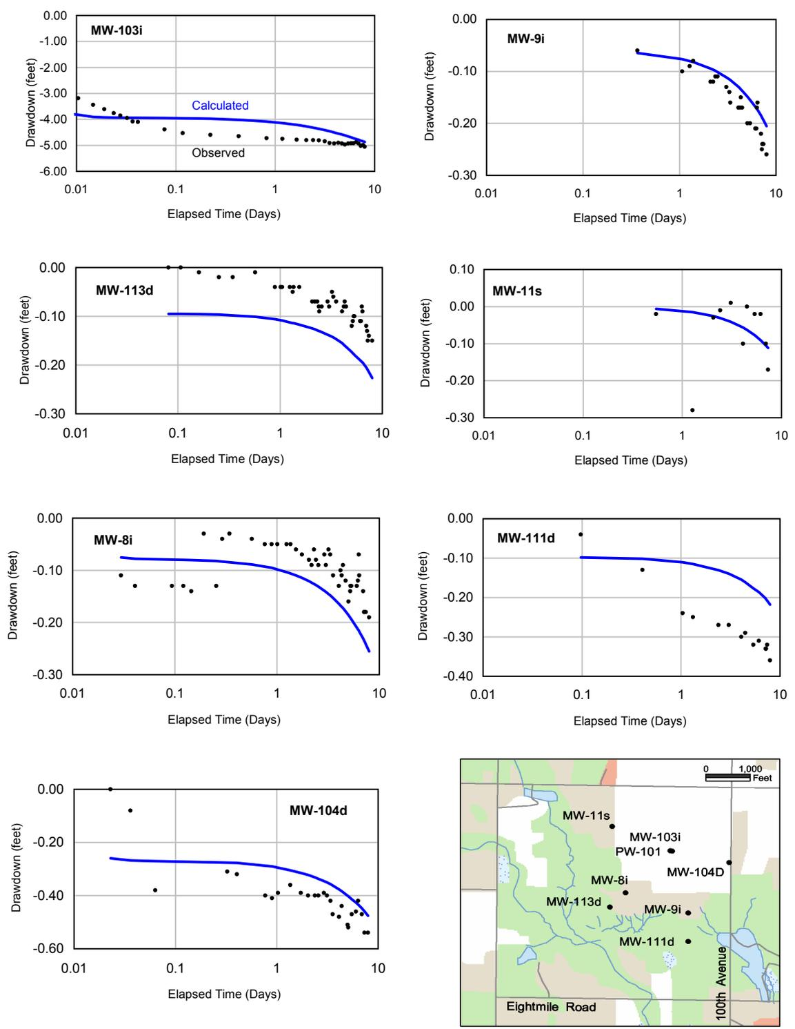
**Note:** PW-101 pumped for eight days at a rate of 400 gpm.
