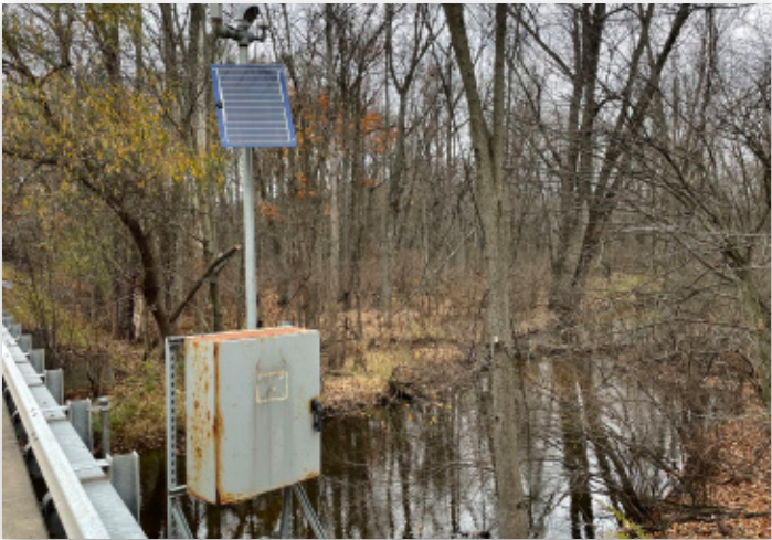
This U.S. Geological Survey gage has collected daily streamflow data for the Pigeon River in Ottawa County since June 2017 at 120th Avenue. Photo courtesy of EGLE.
