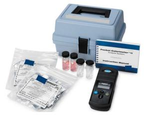
This test kit is more accurate, providing a digital readout of the chlorine residual. DPD is added to the water sample, then the sample is placed into the unit and covered. The unit generates a light that measures the amount of color in the sample and provides the readout.
