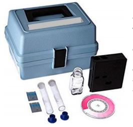
DPD is added to the water sample, then the sample is compared to the color wheel to determine the level of chlorine residual. These kits are quite common due to low cost and ease of use, but are less accurate, depending on the operator's ability to see the pink color and make the comparison. The tubes are also prone to discoloration, and if not replaced on a regular basis, may cause inaccurate results.
