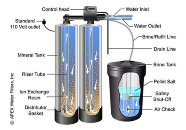
Figure 14.3 Typical Downflow Pressure Type Softener
